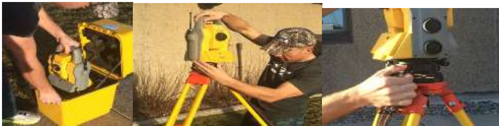
Fig. 2.17setting of tripod on the instrument
