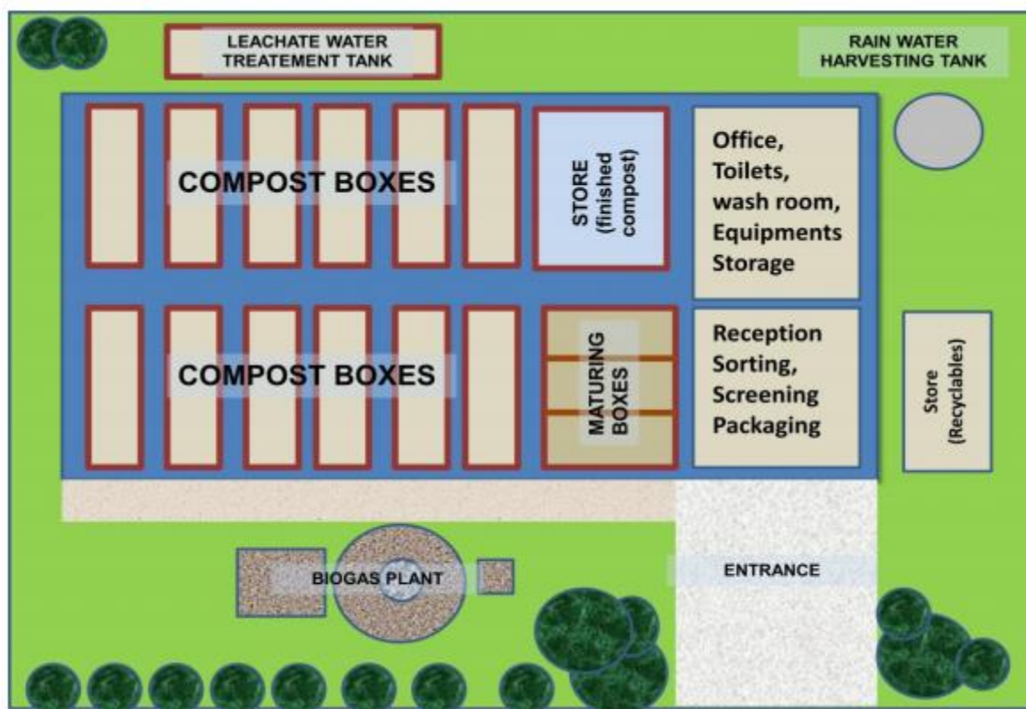
Figure 3.1 Typical schematic layout of box type compost plant
