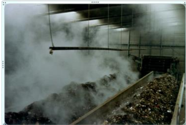
Figure1.6. Composting in rows (agitated by machine), with organic solid waste as a substrate
