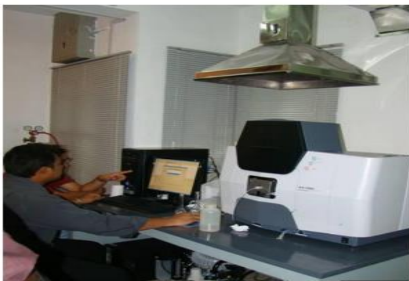
Figure 2.3 an Atomic absorption spectroscopy (AAS) Machine facility for determining heavy metals for compost quality control
