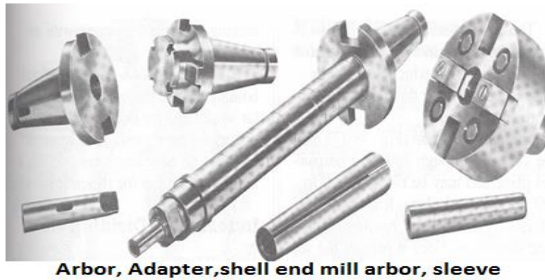
Figure 2.10 Arber, Adapter, Shell end mill Arber, Sleeve
