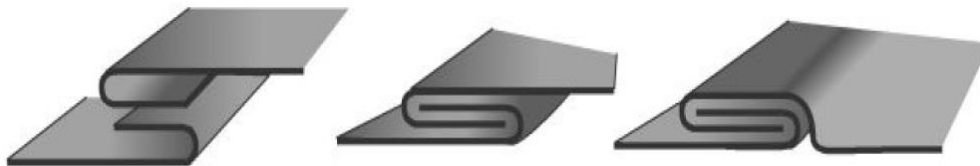
Fig .4.4: Development of a grooved seam joint
