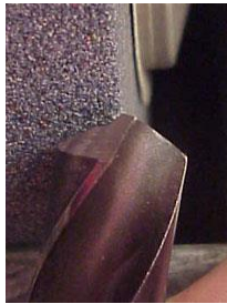
Figure 6.14 Line up the end of the web with the corner of the wheel
