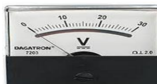
Figure 1. 24 A voltmeter (Analog)
