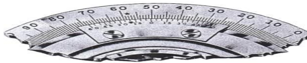
Fig. 6.1.9 Reading the size of an angle of vernier bevel protractor
