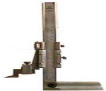
Figure 2.4 Vernier Height Gauge
