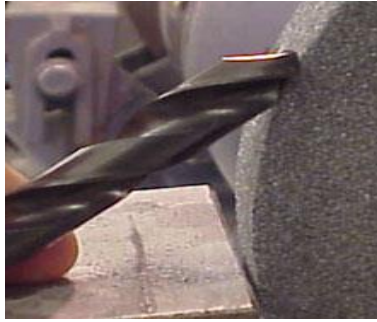
Figure 6.16 approach angle is steeper when web splitting
