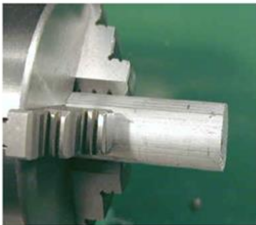
Fig: Facing work on lathe machine
