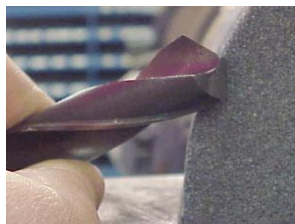
Figure 6.13 Holding the drill at a 30- degree angle
