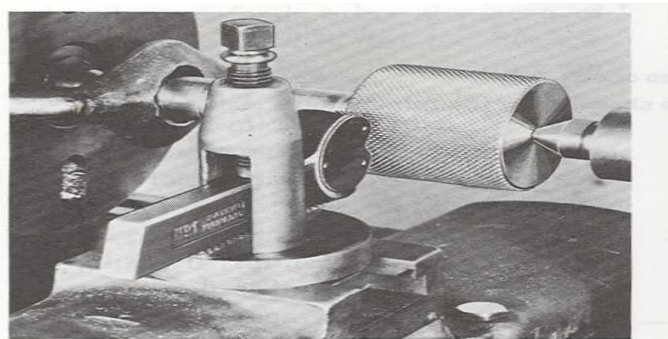
Diamond –point knurling of a cylindrical work piece
