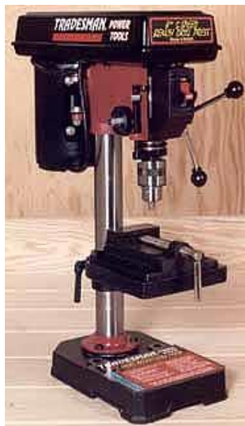
Figure 1.0:5 Pillar Drill Machine
