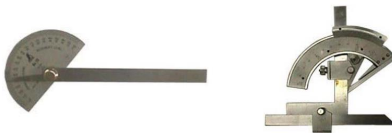
Figure 1412 Engineer's Protractor and Vernier Protractor
