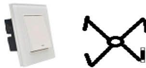
Figure 1. 33 Intermediate switch pictorial diagram and symbol
