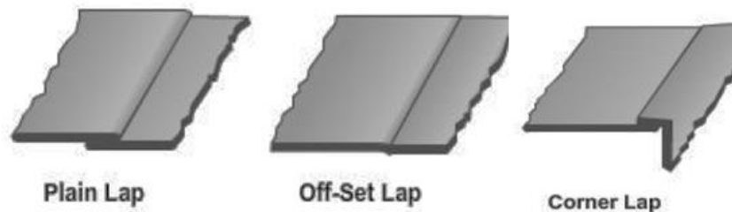
Fig.4.8: Types of Lap seam
