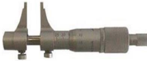
Figure 6.5 Inside Micrometer
