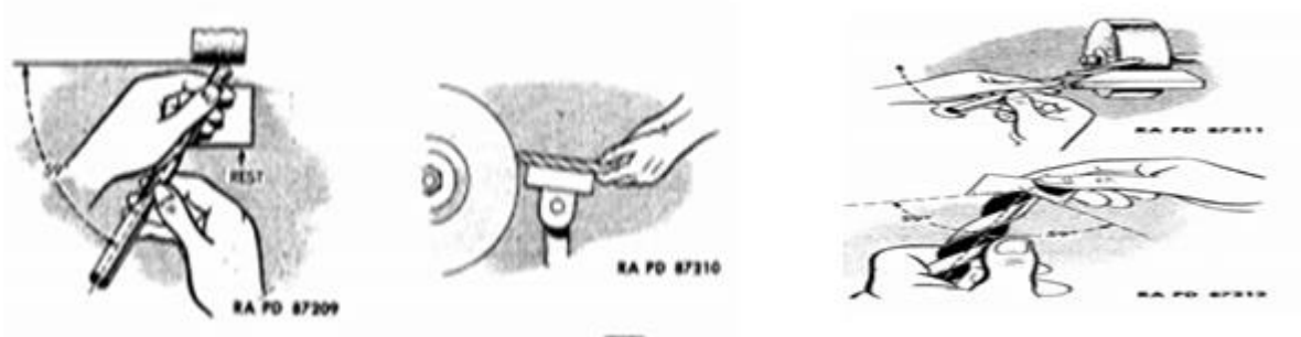
Figure 6.8 Free Hand Grinding
