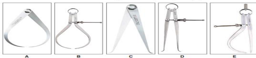
Figure 13 A-firm joint outside caliper. B-Bow spring outside caliper. C-Firm joint inside caliper. D- Bow spring in side caliper. E-Hermaphrodite caliper
