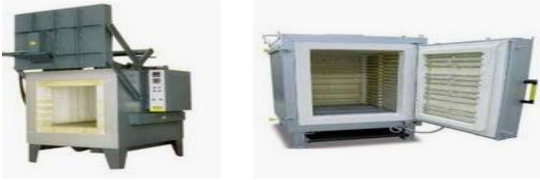
Fig 2.3 Box or box type furnaces
