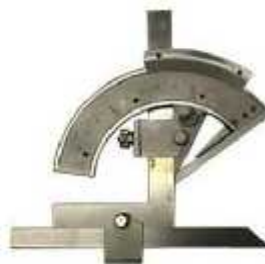
Fig.1.13.Vernier Protractor
