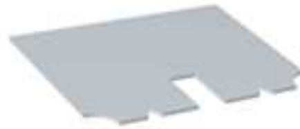
Fig.4.5. Notching operation
