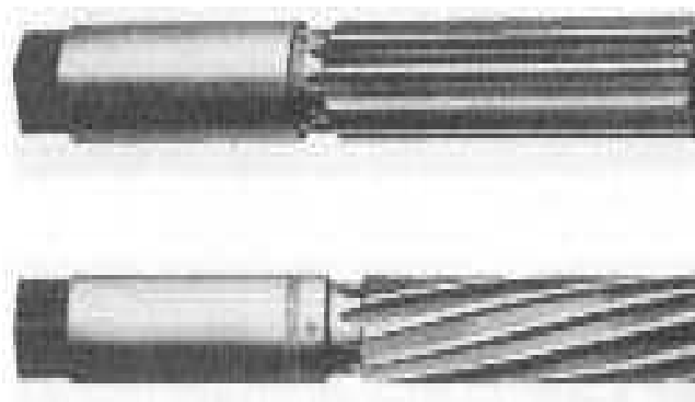
Straight and helical fluted hand reamers
