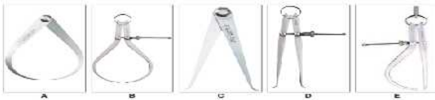
Fig. 1.11 A. Firm joint outside caliper .B. Bow spring outside caliper C. Firm joint inside caliper D. Bow spring in side caliper. E. Hermaphrodite caliper
