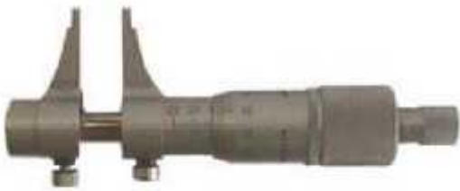
Fig.1.5. inside Micrometer
