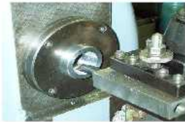
Fig4.3. Boring operation.
