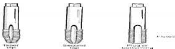
Figure 4.18 Taps for cutting internal threads.
