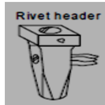
Fig1.14. Rivet header
