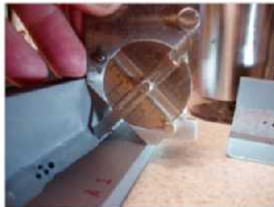
Figure 3.11. Throat measurement with cam gauge
