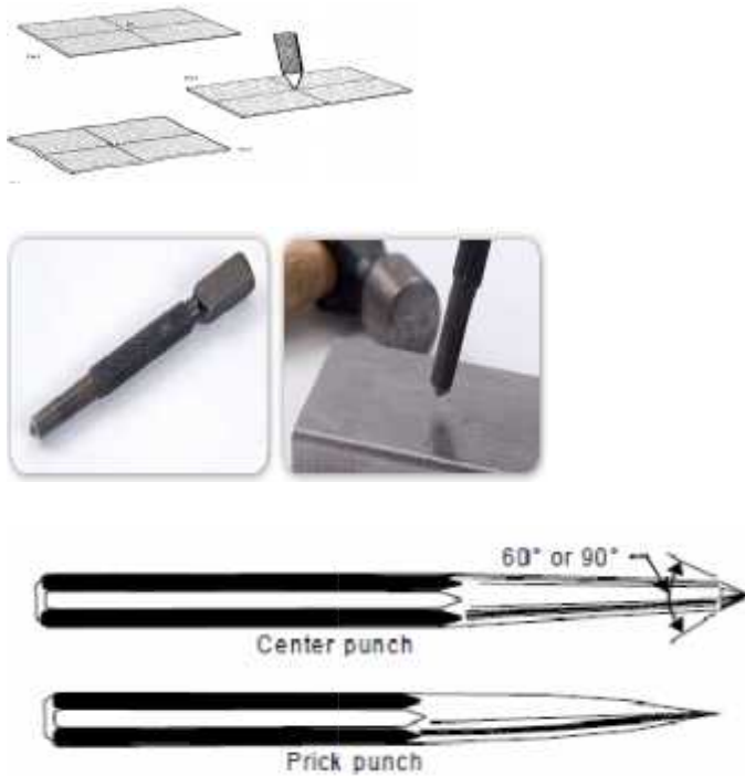
Fig.1.20. A Center punch and the punch in use.
