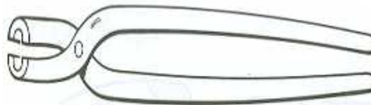
Figure 1.13.Hollow bit tong
