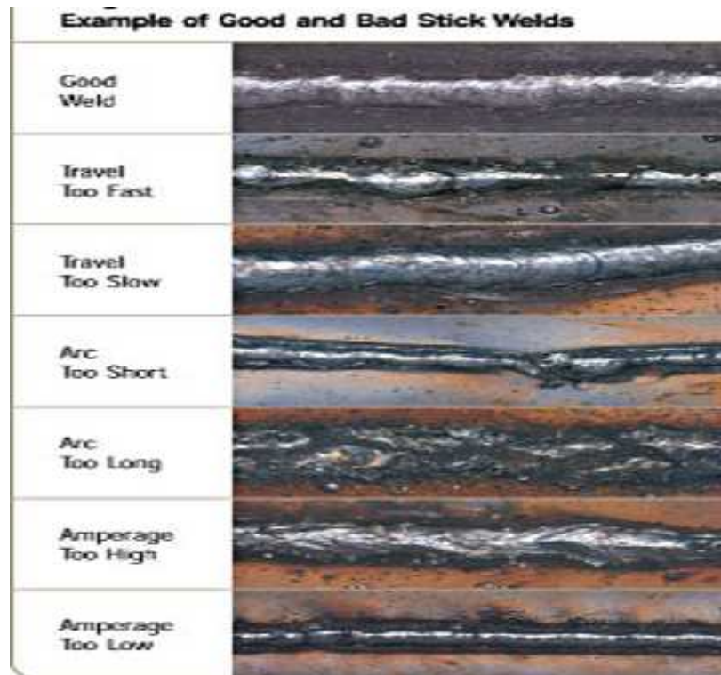
Figure 2.1.Effects of the major weld parameters: speed, current and arc length
