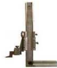
Fig.1.18.. Vernier Height Gauge
