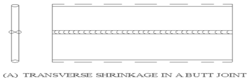
Fig.2.19. Transverse Distortion
