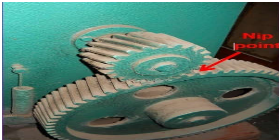
Figure 1.4. Dangerous parts of machinery on gear wheels. Between rotating and tangentially moving parts
