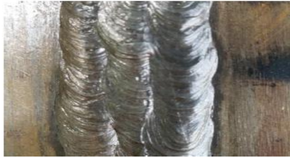
Fig5.2. Fusion on weld face and toes
