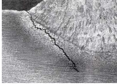
Fig.3.1. Cold cracks
