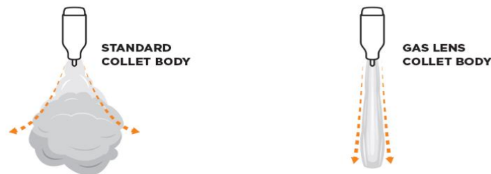
Fig.2.5. Lens vs. Gas lens
