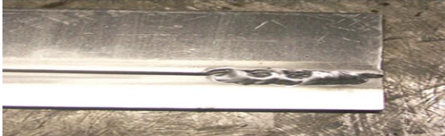
Fig.2.13. cause of Excessive voltage on a Control of the weld pool.
