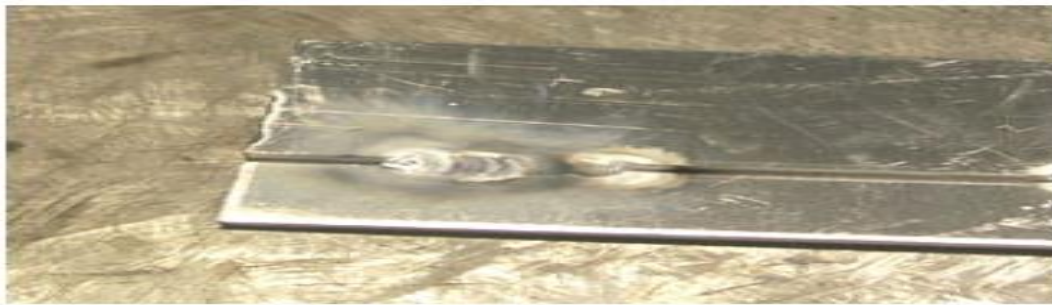
Fig. 2.14. Cause of insufficient voltage on the electrode to stick.
