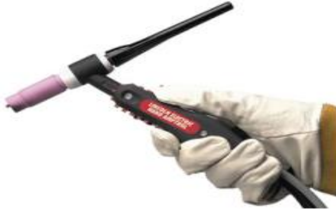
Fig.2.11. use of torch with a hand to control current levels.
