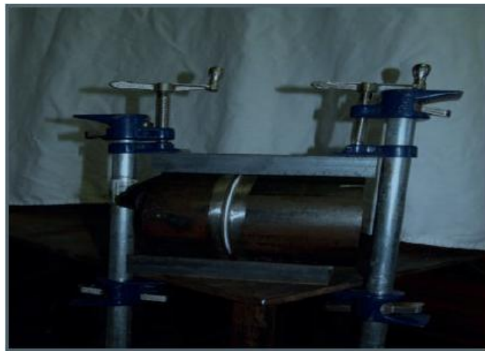
Fig.1.8 Channel Iron Used for alignment.
