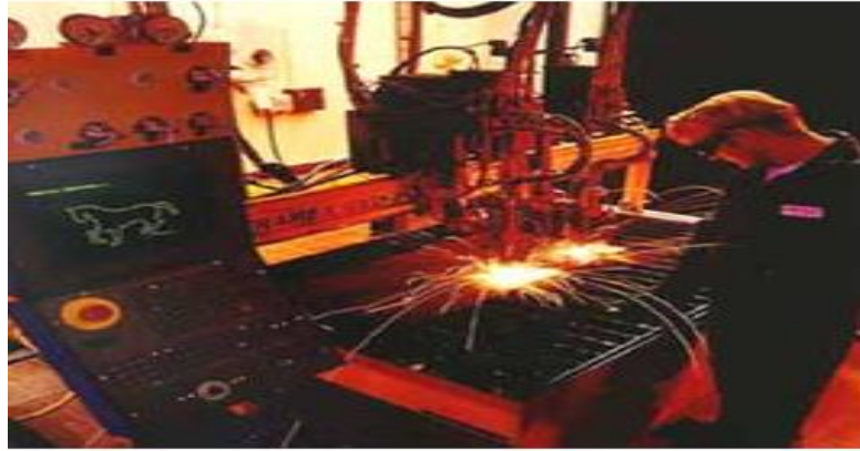
Fig.3.9. Mechanized oxyacetylene cutting system
