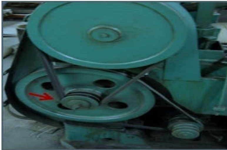
Figure 1.5. Dangerous parts of machinery on belt drives.
