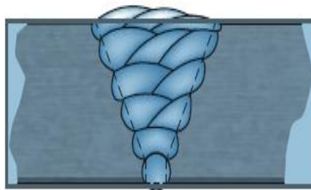
Figure: - 4.1.1.1 Weld layers in groove weld.
