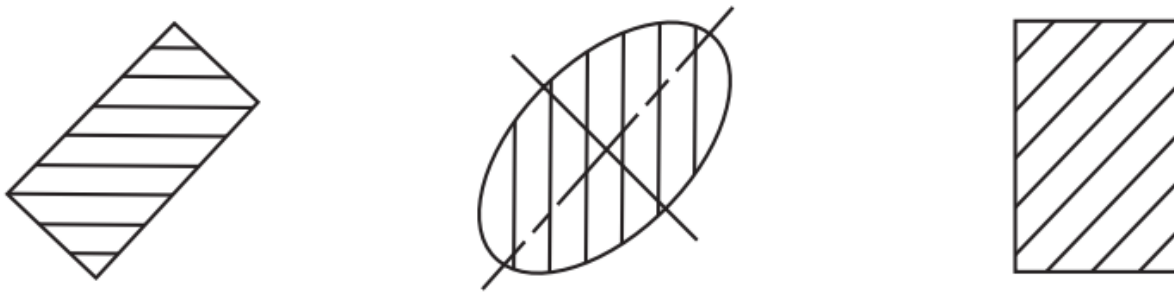
Figure 2.10 Preferred hatching angles
