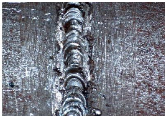
Fig 5.1 Fusion on the root side-both beveled pipe edges are melted.
