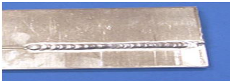
Fig.2.12.Narrow welds in GTAW.
