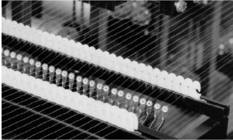
Figure 1.16: Yarn break sensors
