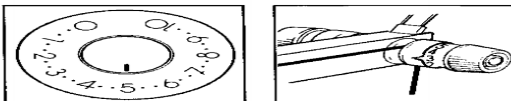
Fig. 42 Tension dial and stitch dial
