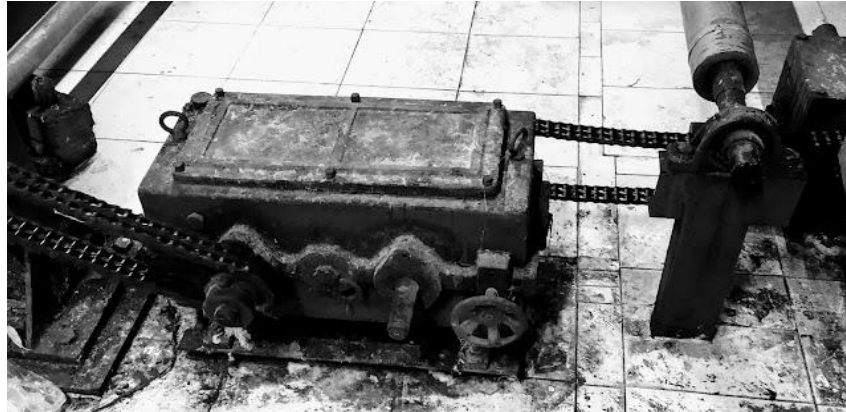
Figure 3.13: PIV gearboxes
