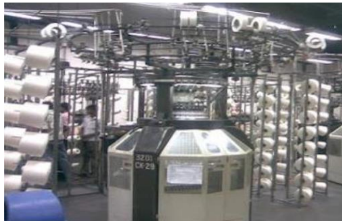
Figure.1.10: Creel of Circular Weft Knitting Machine
