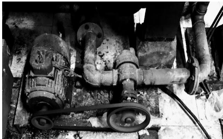
Figure 3.8: Liquor circulation system
