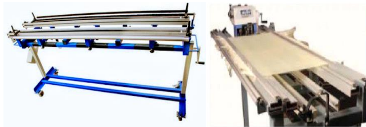
Figure 2.2: Dressing of warp sheet
