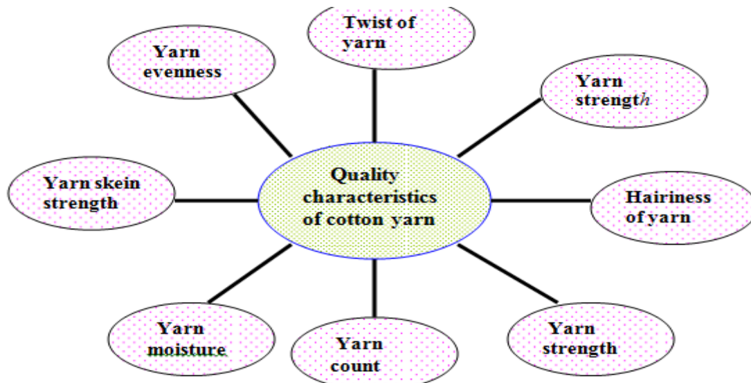
Fig 10 Quality characteristics of yarn
