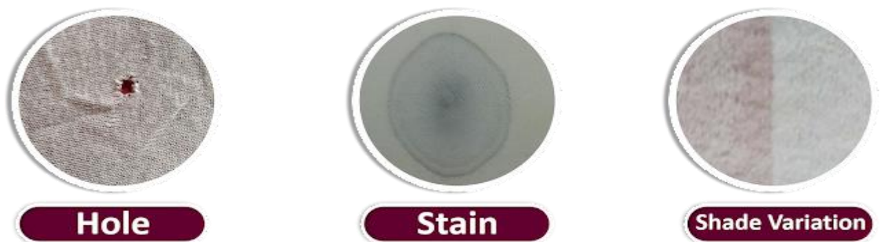
Fig 48 Defects from Machine Setting
