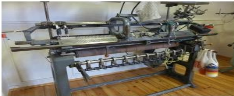
Fig.2 Straight bar frame machines
