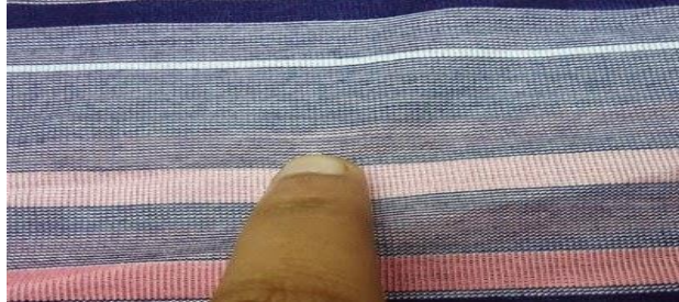
Fig 49 barrier fault
