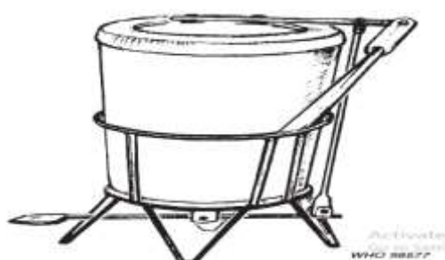
Cylinder-type waste container made from oil drum cut in half
