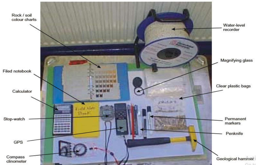
Figure 4. Equipment required for collecting and analyzing data during drilling
