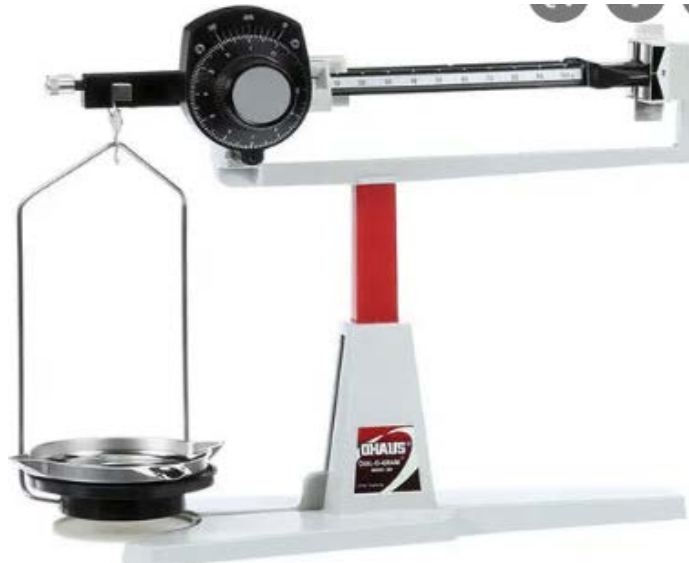
Figure 3.1: Dial - O - Gram Mechanical Balance
