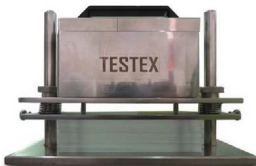
Figure 6.2: Perspiration tester
