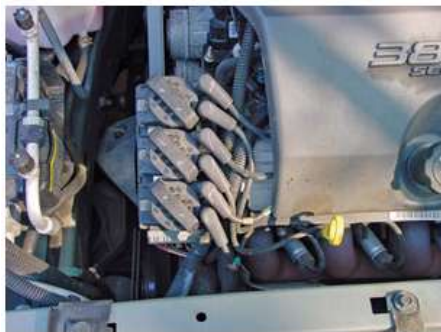
Figure 1.3-22A coil pack for a double-ended waste spark ignition system or Figure 27–24 A coil per cylinder ignition system
