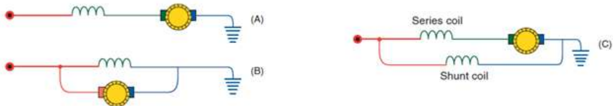
Figure 1.2-14 Starter motors are grouped according to how they are wired: (A) in series, (B) in parallel (shunt), or (C) a compound motor using both series and shunt coils.
