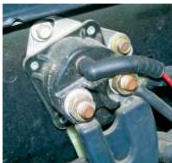
Figure 1.2-19 Starter relay/solenoid mounted on a vehicle.
