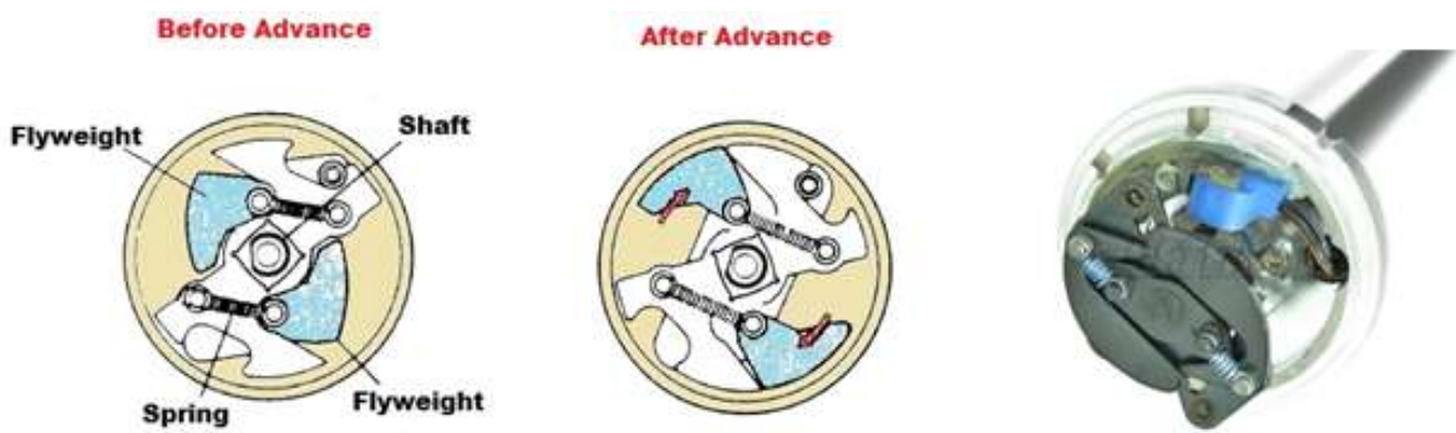
Fig 1.3-8 Centrifugal-advance mechanism
