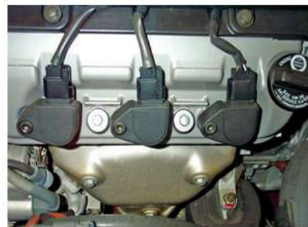
Figure 1.3-22A coil pack for a double-ended waste spark ignition system or Figure 27–24 A coil per cylinder ignition system
