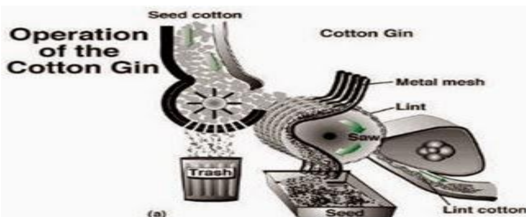
Fig:6 Operation Principle Of Gin Stand
