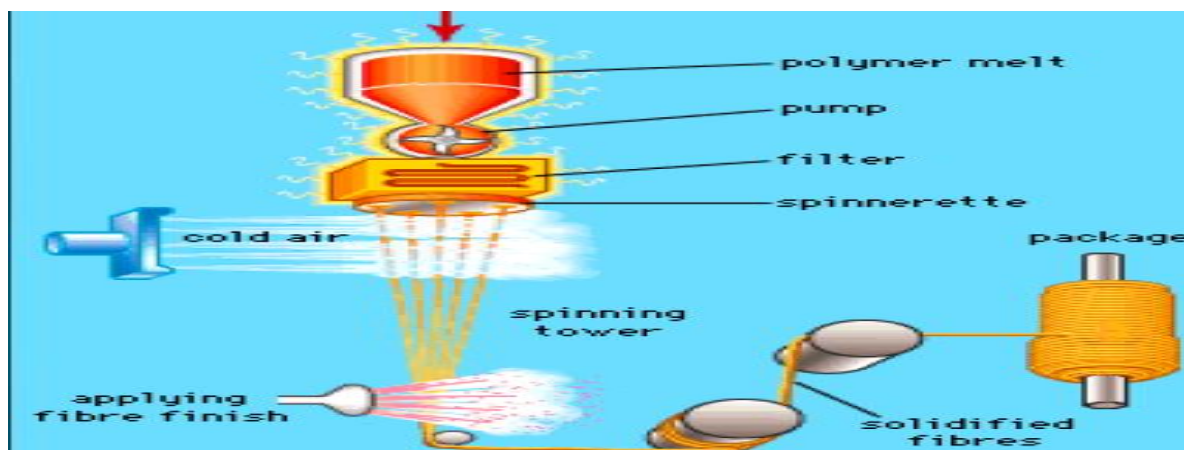
Fig: Principle of Melt spinning
