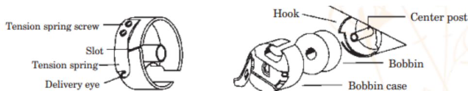
Fig:- 1.3.28. Bobbin case and bobbin mechanism
