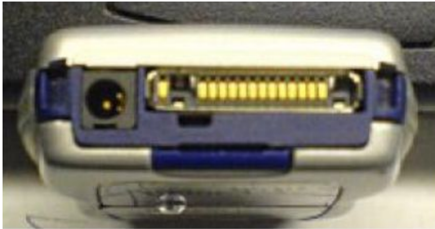
Fig 4.9 Nokia 3220 Fbus connections (Harrington 2007)
