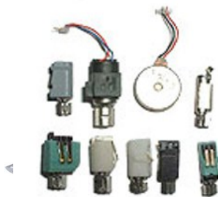
Fig.3.8 Shows Buzzers and Ringers
