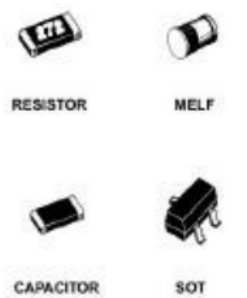
Fig 5.6 - Common discrete SMT components
