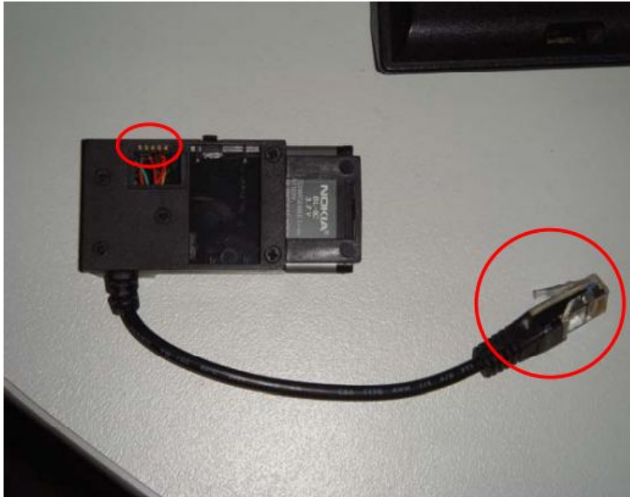
Fig4.8 Connectors on the UFS3 cable for Nokia 6600
