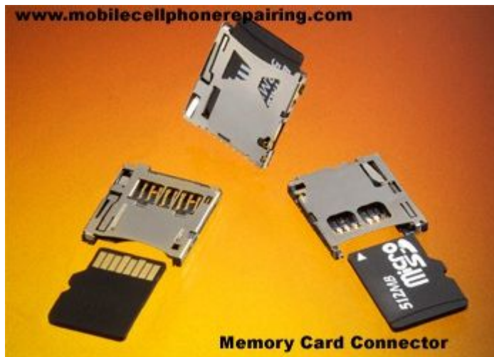
Fig.3.17 Shows Mobile Phone Memory Card Connector
