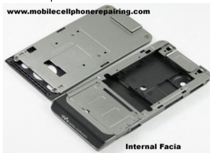
Fig.3.3 Shows Internal Facia or Skeleton of a Mobile Phone
