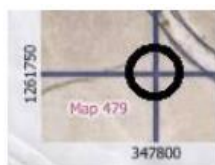
Fig. 3.5. Easting 347800 and Northing 1261750 for a grid cross.
