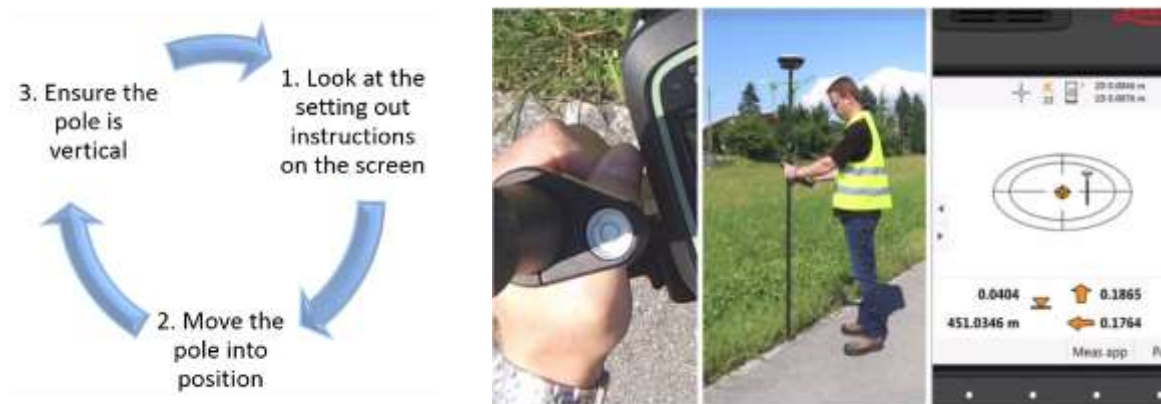
Fig 3.1 Simplified setting out with GNSS/GPS instrument
