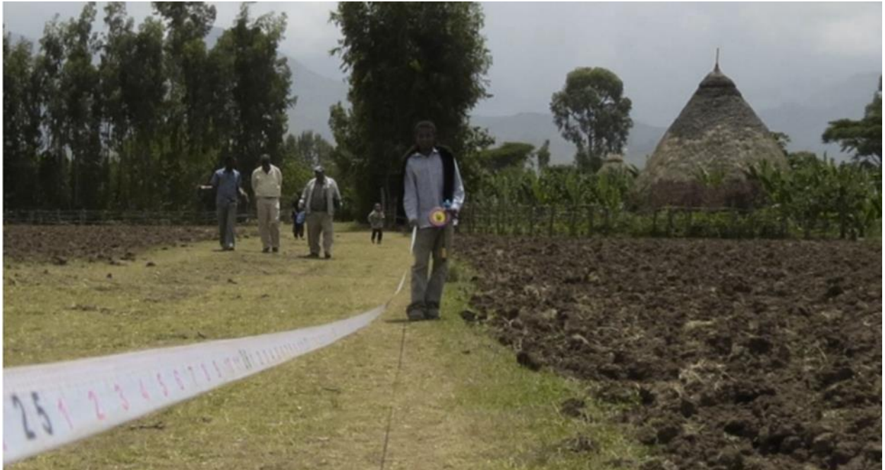
Fig. 2.2. Tape measurement
