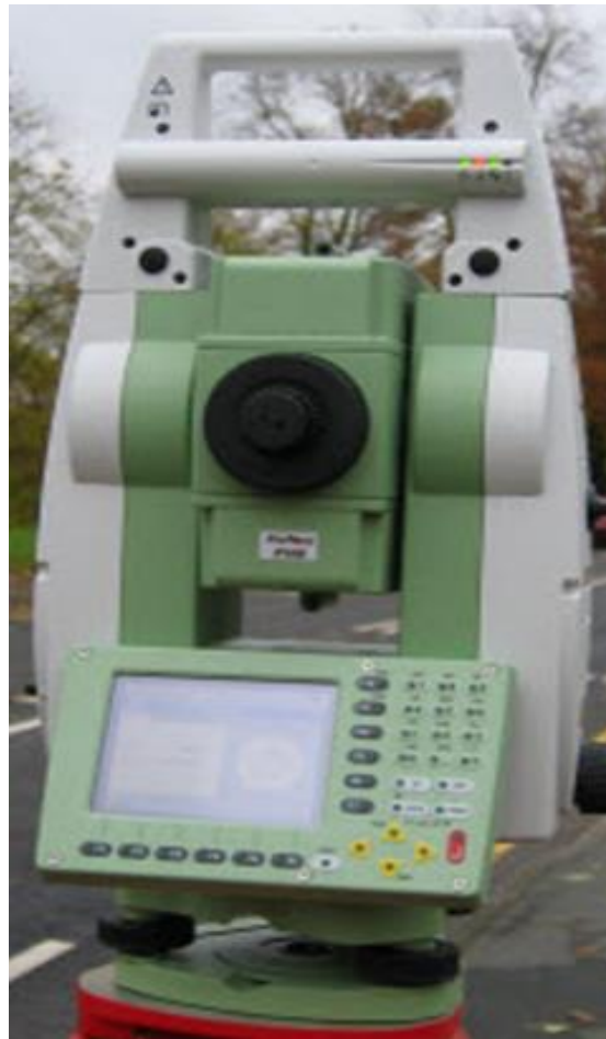
Figure 1.6 Leica 1200 total station
