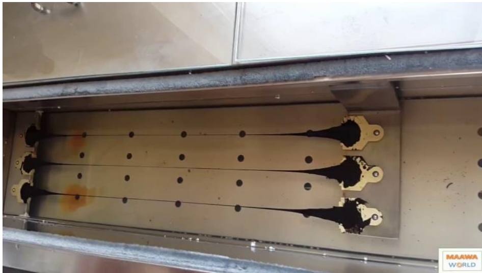
Figure 2-6 Ductility Test:
