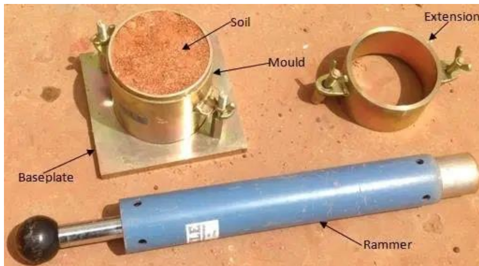
Figure 2-2 Compaction Test
