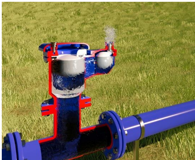
Figure 3. 23 Air release valves
