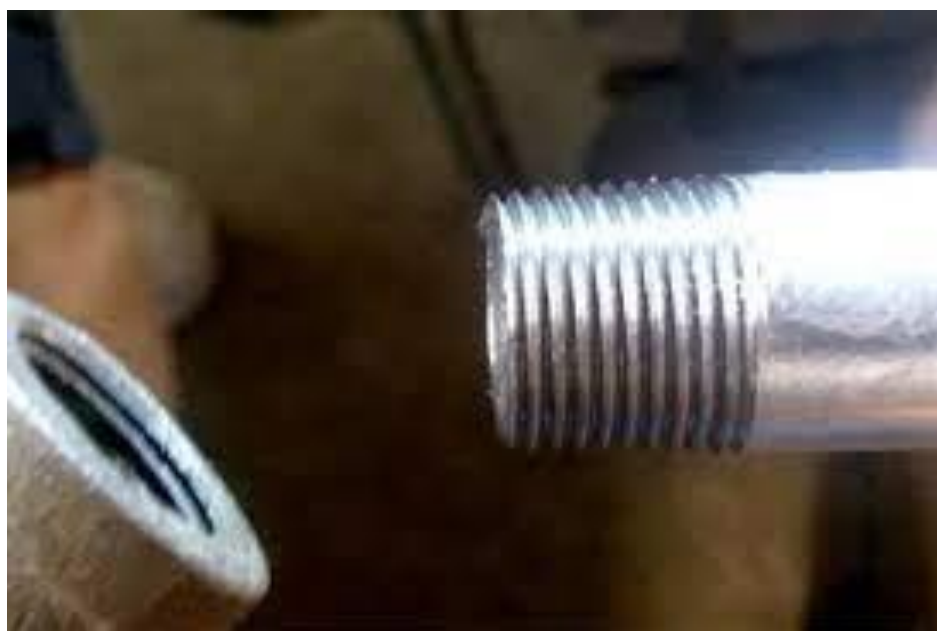
Figure 3. 16 Threaded joints
