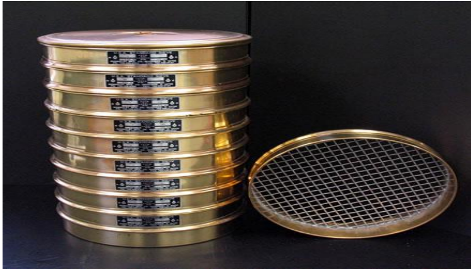
Figure 2-1 Gradation Analysis test
