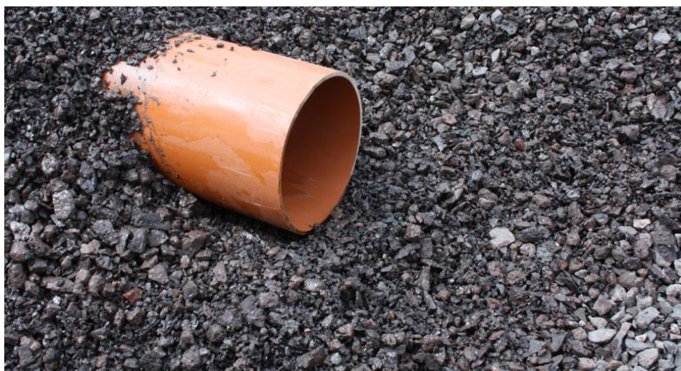
Figure 2. 20 Pipe bedding
