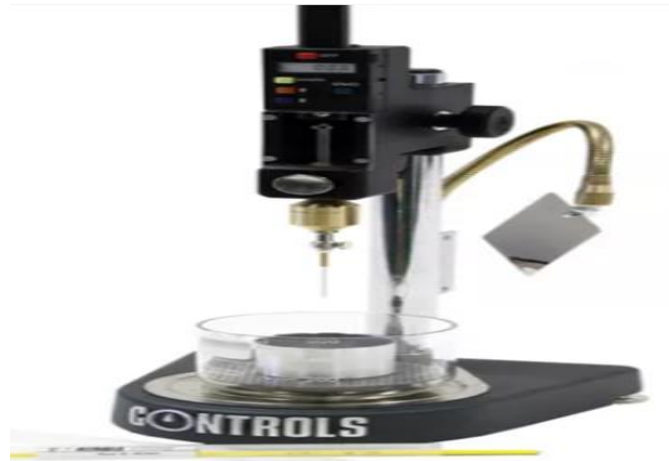
Figure 3-3 Bitumen Penetration test equipment
