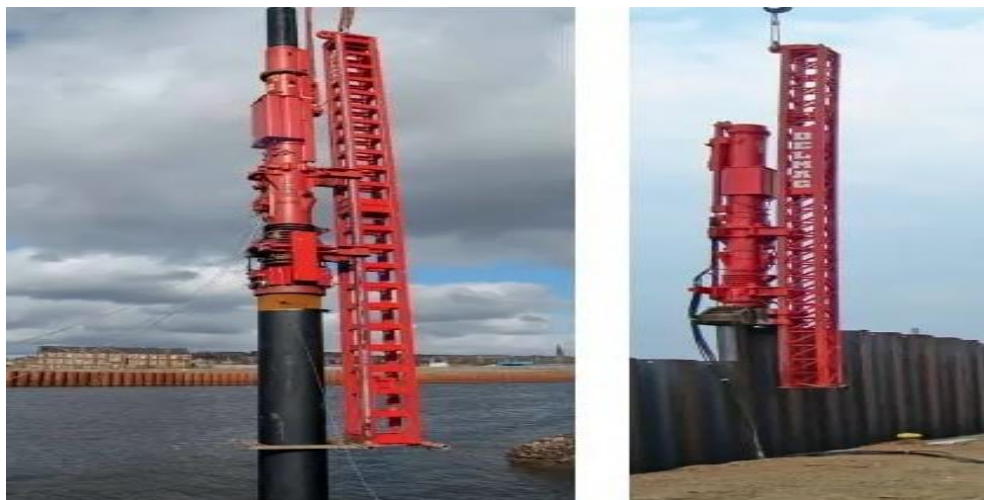
Figure 4-3 Hammer Guided and Rope Suspended Leader
