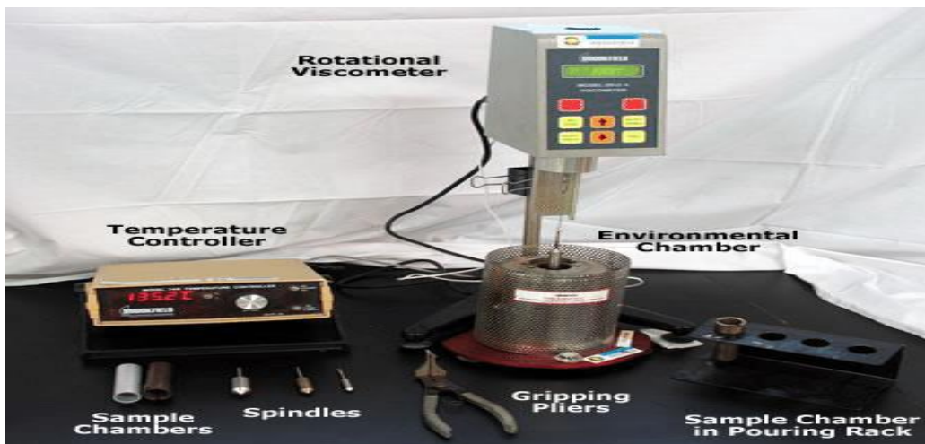
Figure 2-8 Viscosity Test of Bitumen
