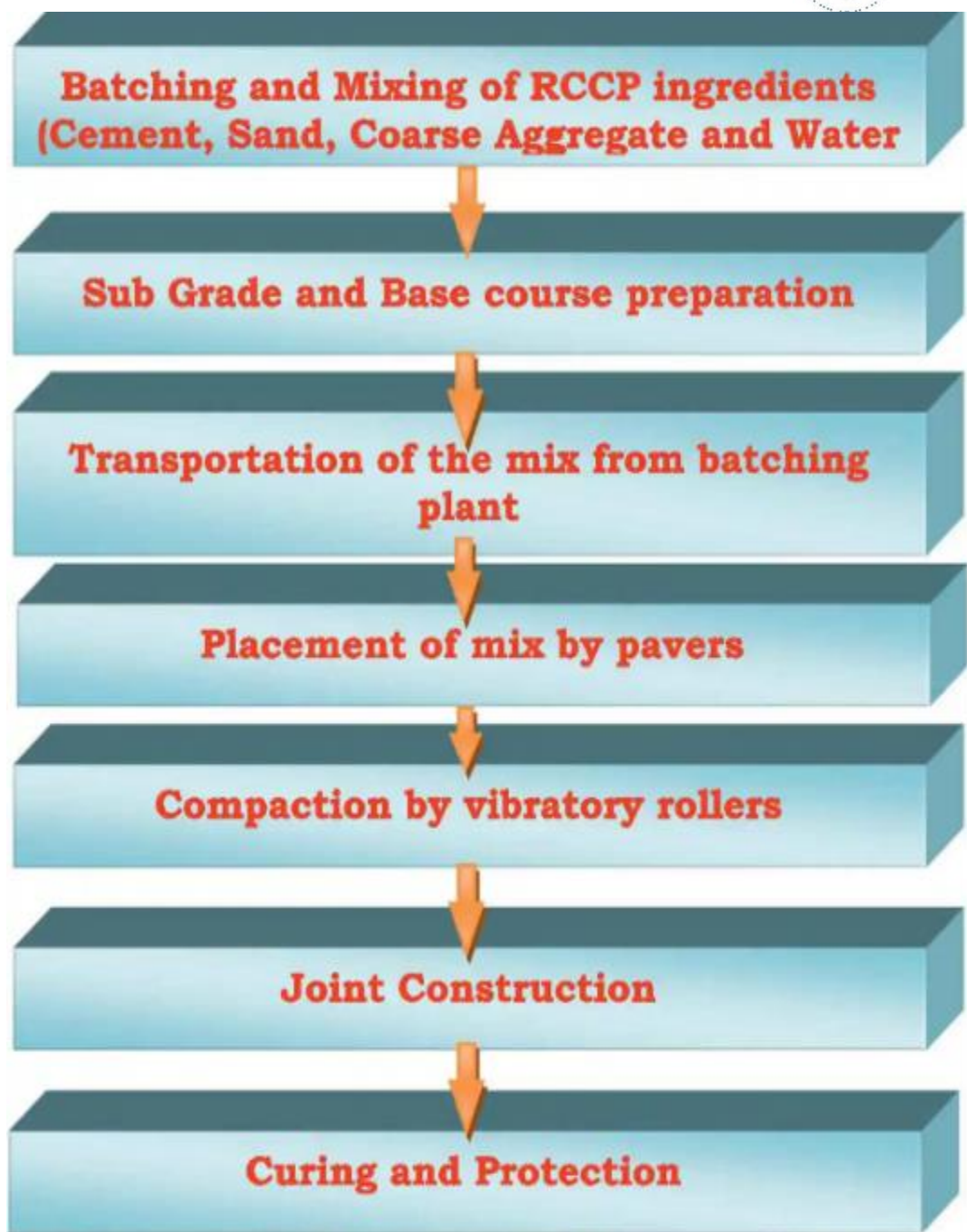
Fig1.53. Roller Compacted Concrete Pavement
