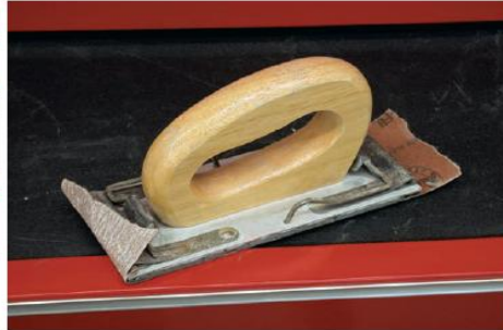
B A short sanding board is needed to level and smooth body filler on smaller repair areas.
