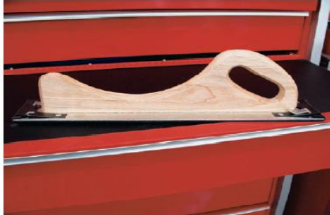
A A long sanding board will quickly level and smooth large areas of body filler on flat body parts being repaired.
