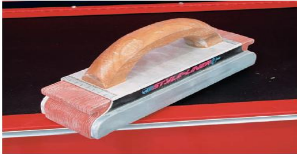
A The sanding block has movable parts that can be moved to match shape of body panel.
