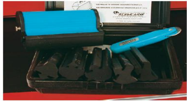
FIGURE 4-79 This sanding block has interchangeable shapes. You can select a shape that matches body panel to repair complex body lines.
