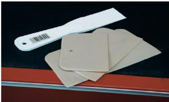
FIGURE 4-80 Upper left, a plastic putty knife should be used to mix body filler and hardener. Lower right, spreaders are used to apply body filler after mixing.
