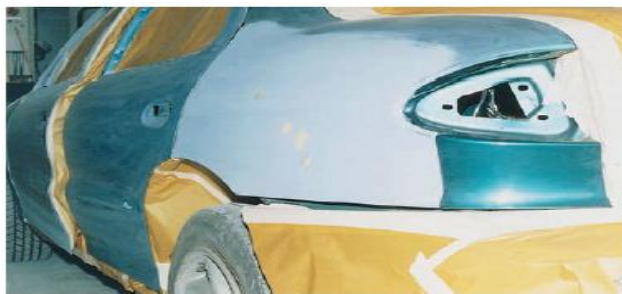
FIGURE 25-21 This quarter panel has been straightened, body filled, primed, and spot puttied. It is now ready for final fine sanding to prep it for topcoats of paint.
