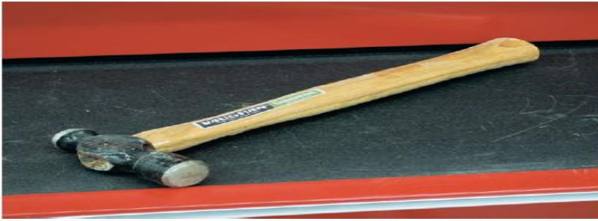
A The flat head is for hammering on flat surfaces and the round head is for concave surfaces.
