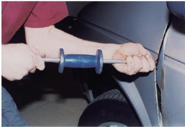
FIGURE 4-61 Here the technician is using a slide hammer to pull out and straighten the bent edge of a front fender.
