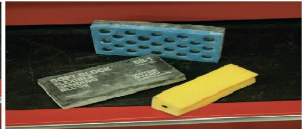
B Thin, soft sanding blocks are used for final sanding.
