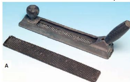
FIGURE 4-71 A body file is often used to rough cut high spots in body filler after partial curing. This saves sanding time and does not produce sanding dust. Large teeth in the body file will scrape off semi-hard body filler quickly and easily.
