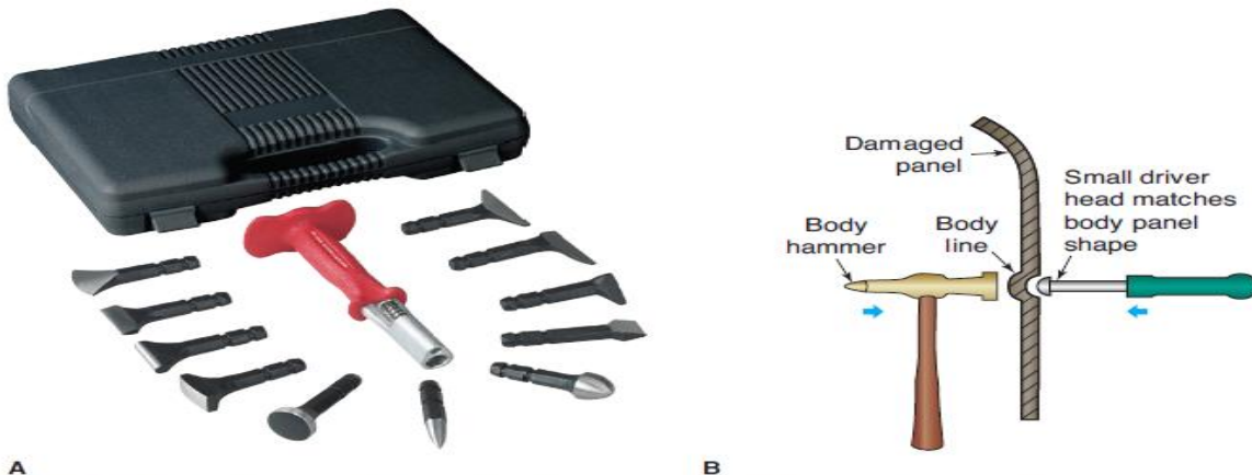
FIGURE 4-54 An interchangeable driver set is handy because you can match the shape of the driver to the desired contour of the sheet metal panel being straightened. (A) Note the different driver heads that can be used to reshape and fix damaged sheet metal. (B) A small driver head can be placed into a dented body line to hammer it straight quickly. (Courtesy of SPX/OTC Service Solutions)
