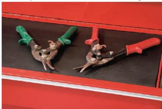
A Sheet metal cutting pliers come in right- and left-hand configurations for cutting in different directions.
