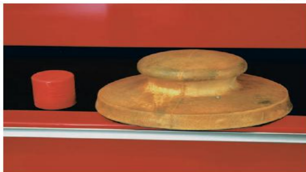
FIGURE 4-75 The size of the sanding block must match the job. On the left is a tiny sanding block for repairing minor dirt damage in freshly applied paint. On the right is a large round sanding block that will accept Velcro-type sanding discs.
