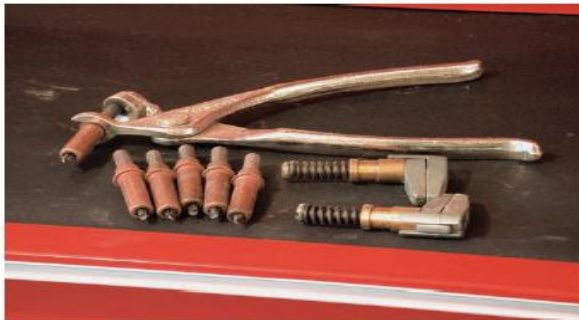
A These spring-loaded rivets and clamps can be installed and removed easily using special pliers. (Courtesy of Eastwood Company, www.eastwood.com )
