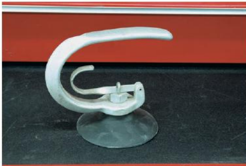
FIGURE 4-62 This hand-held suction cup tool will grasp and pull on glass or smooth body panels.
