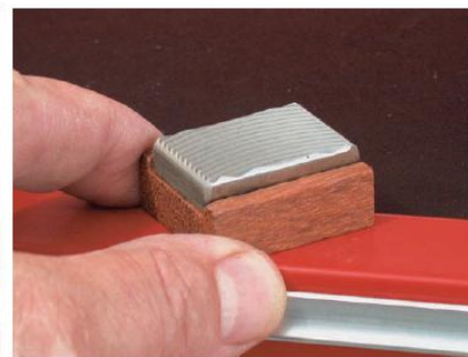
FIGURE 4-72 A dirt nib file is a small, finger-held tool used to carefully cut off dirt and dust particles in new paint.
