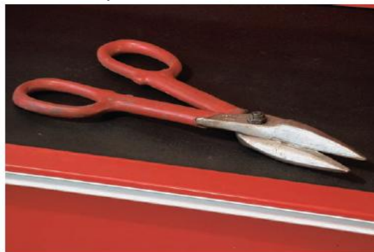
B Straight-jaw sheet metal cutting pliers are handy when you have plenty of room for cutting.
