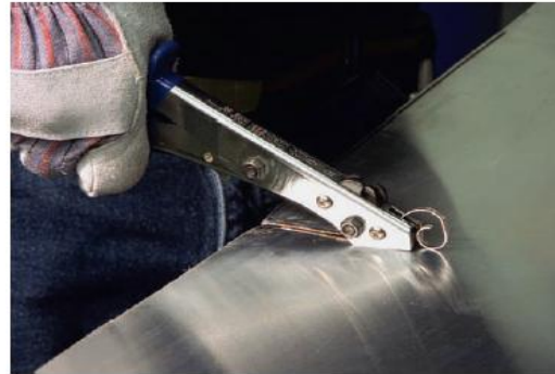
B The center jaw pinches between two stationary jaws to shear a thin strip of sheet metal away for cutting. (Courtesy of Eastwood Company, www.eastwood.com )
