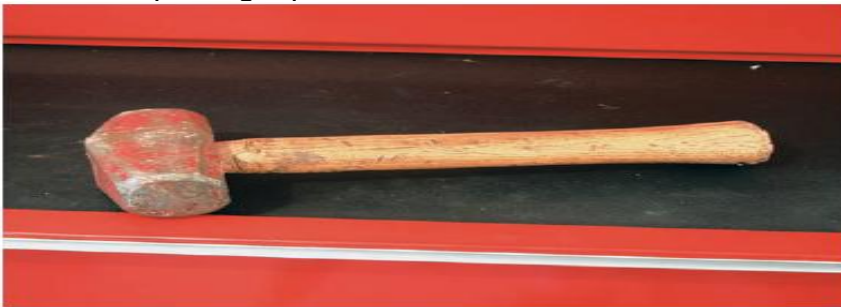
FIGURE 4-45 The heavier mini-sledge hammer will produce a much more powerful blow than a small hammer.
