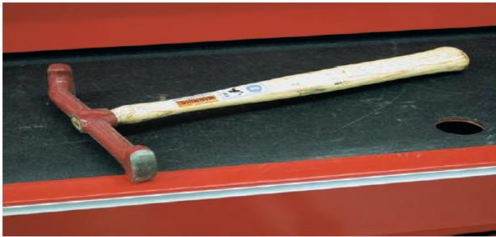
FIGURE 4-50 This body bumping hammer has a very large, long head on it for working obstructed areas on damaged panels.
