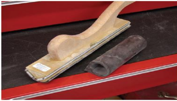
FIGURE 4-77 Again, the sanding blocks should match the shape or contour of the panel being repaired. On the left is a rounded sanding board for shaping long, curved body lines. On the right is a round rubber sanding block for shaping smaller curved surfaces.
