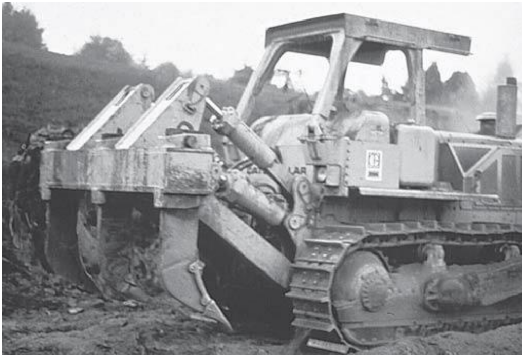
Figure 4-8. Tractor with a hydraulic ripper attachment.
