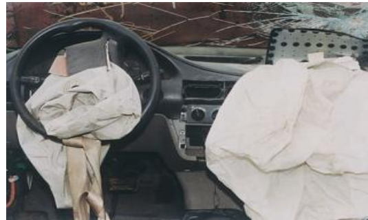
Figure 2 Lamination kept this windshield glass intact upon impact. Tempered glass would have shattered into small pieces. Air bag deployment often shatters windshield glass.
