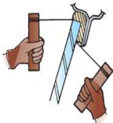
FIGURE You can cut through windshield adhesive with Piano wire. Be extremely careful not to cut your hand!
