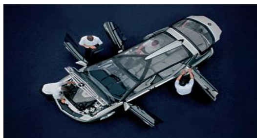
Figure 1 The doors and glass are important structural members in a modern vehicle. They must be serviced properly for the driver and passengers to be safe while driving.
