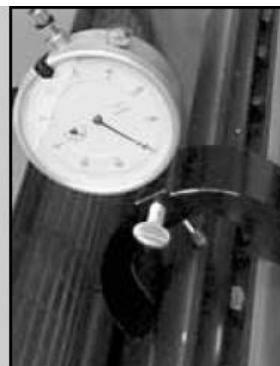
Dial-gauge micrometer for knife alignment - # 30-050
