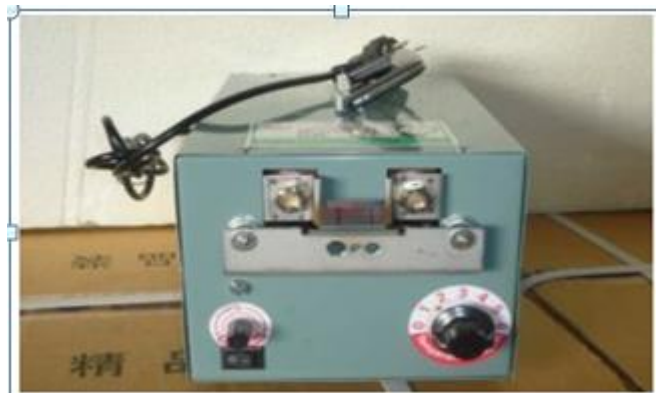
Figure 2: Automatic beak trimming machine
