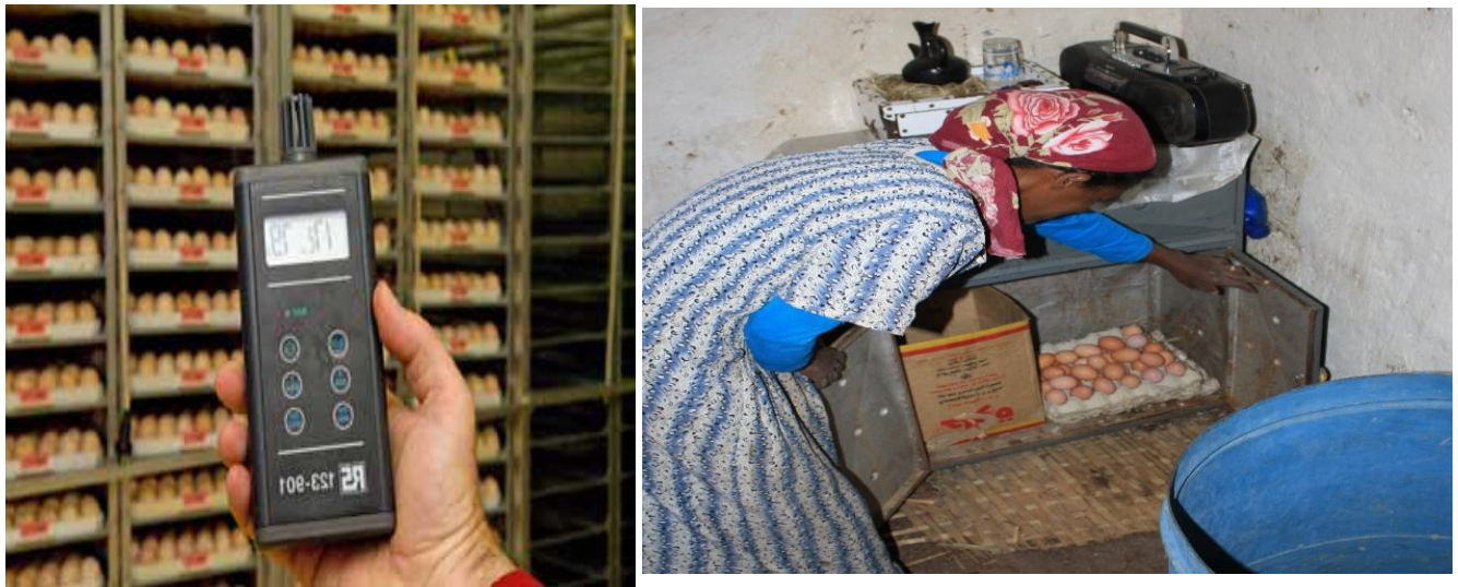
Figure-6, checking egg store environment using a temperature and humidity sensor.
