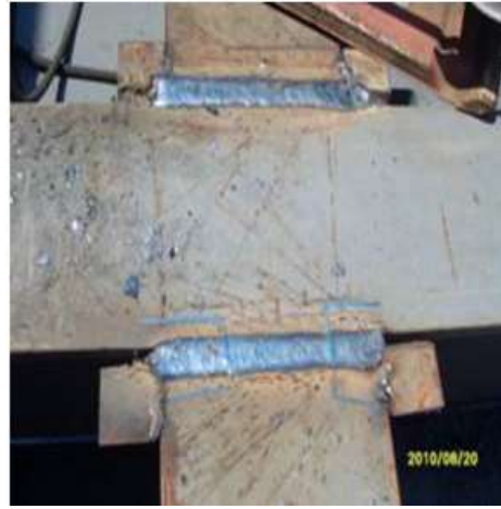
Figure 129 Missing Tab Piece
