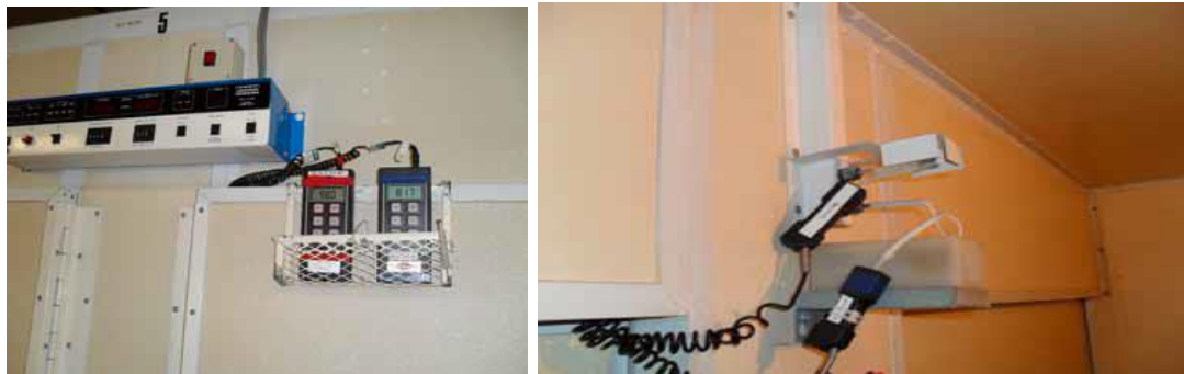
Figure 6 Calibrating by locating the calibration probe next to the machine temperature sensor
