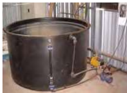
Figure 2.1. A single tank injection system based on a centrifugal pump.
