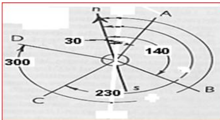
Figure 2.9 Whole circle bearing
