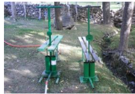
Figure 2.16: Treadle pump
