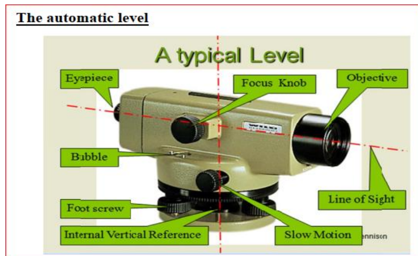
Figure 3.2 Automatic level and their head parts
