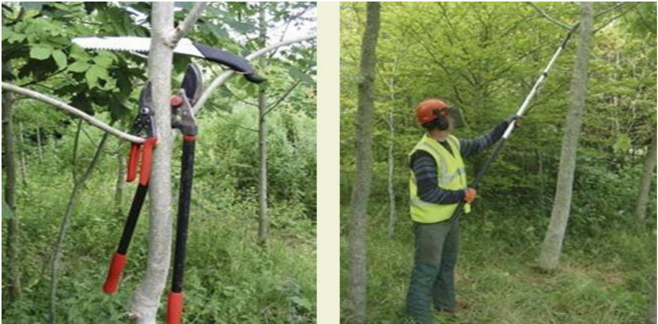
Figure 3.2 Secateurs, loppers and pruning saw (left) and telescopic pruning saw (right)
