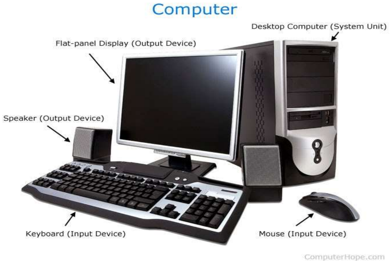
Fig 1.1: Basic parts of computer
