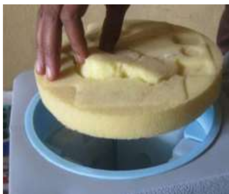
Fig 2: Foam pad cuts to hold vaccine vials
