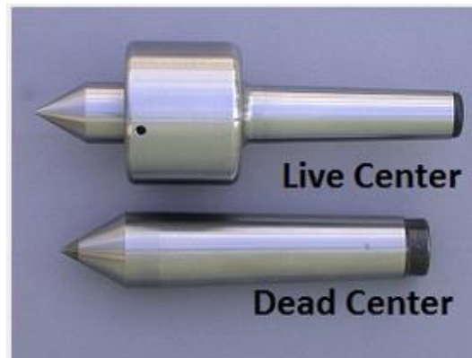
Figure 3.9 Centers adjusting
