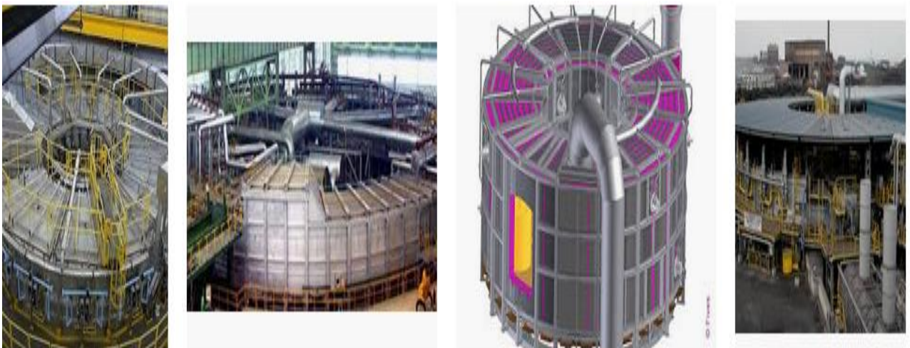
Figure 3.5 Rotary hearth furnace
