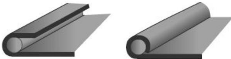
Figure 2.5.Development of a wire edge on a cylinder
