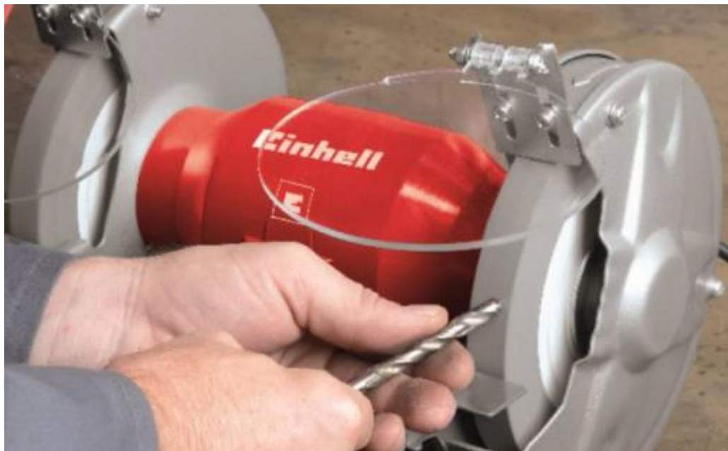
Figure 3.6 Drill bits sharpening.
