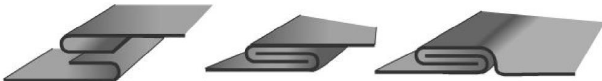
Figure 2.6.Development of a grooved seam joint
