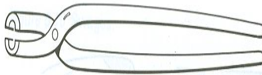
Figure 1.13. Hollow bit tong
