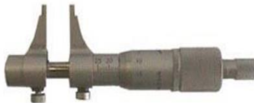
Figure 3.7 Inside Micrometer
