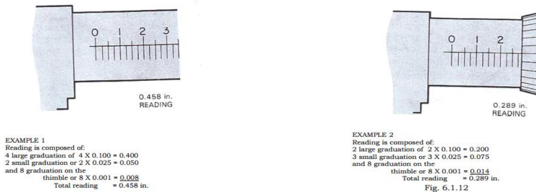
Figure 2.6 Reading micrometer
