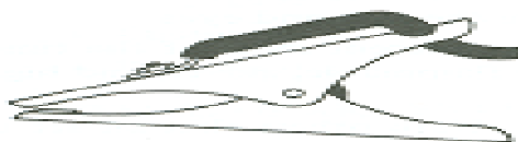
Figure 1.22. Ground clamp
