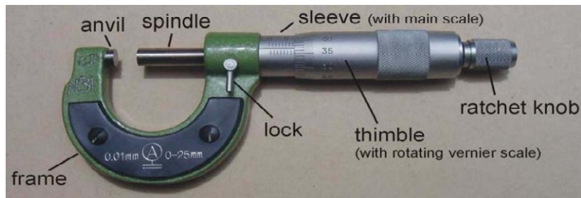
Figure 2.4 outside micrometer
