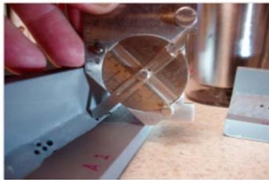
Figure 3.11. Throat measurement with cam gauge
