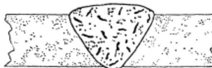
Figure 3.14. Slag inclusion
