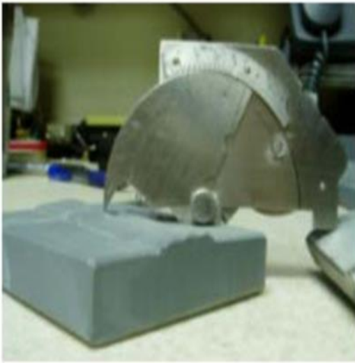
Figure 3.14. Measuring weld Reinforcement
