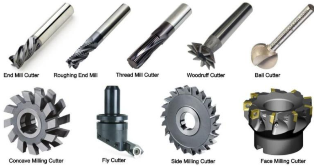
Figure 3.3 Milling cutting tools
