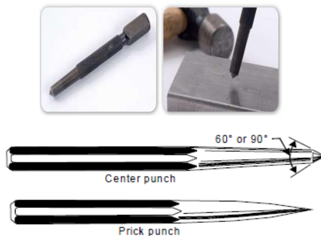
Figure 2.19. Center punch, and the punch in use.
