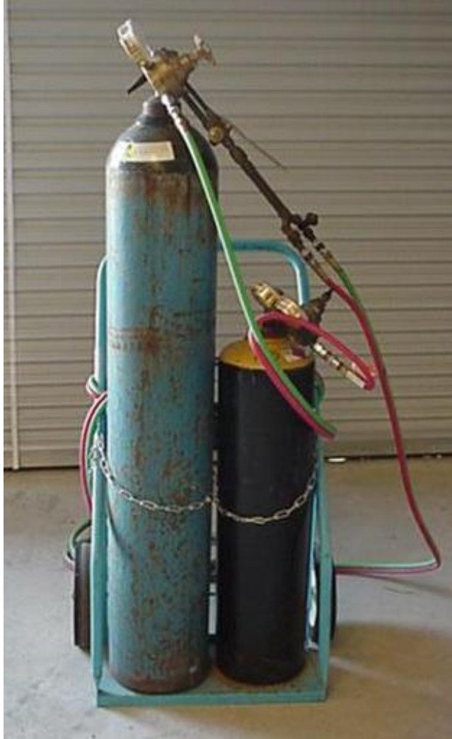
Figure 3.3. Assembled oxy acetylene cutting out fit
