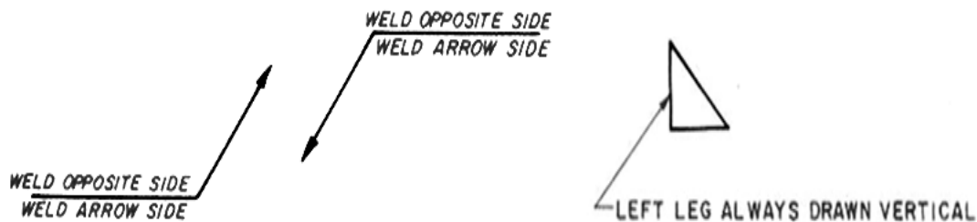
Figure 2.3. Fillet weld symbol
