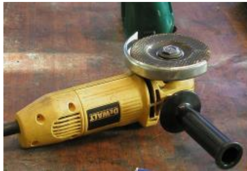
Figure 2.3 Portable or hand grinding machine
