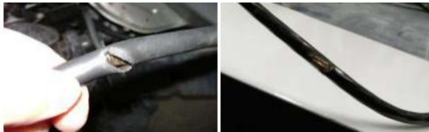
Figure 2.9 Look for tear/cut insulator
