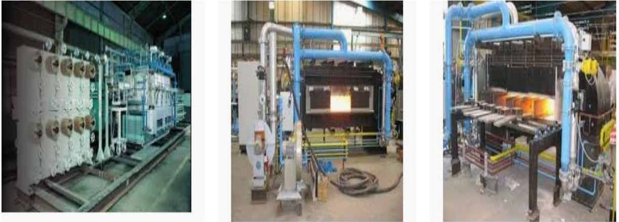
Figure 3.4 Slot type furnace
