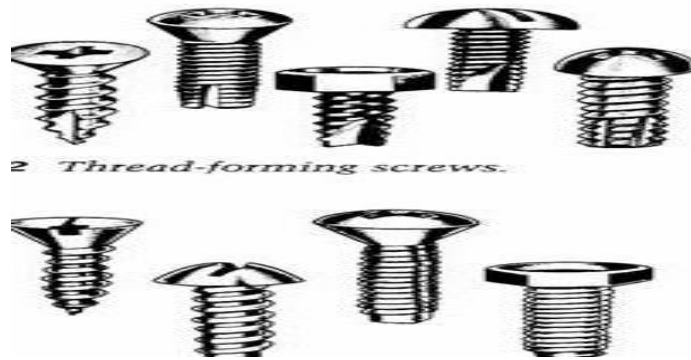
Figure 3.5. Thread cutting screws
