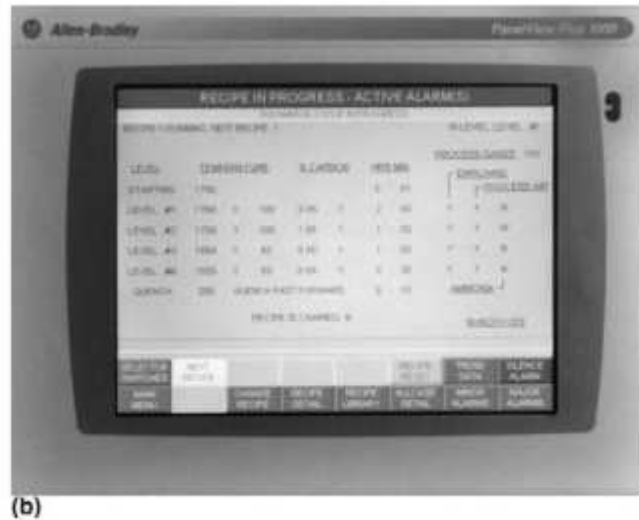
Fig.2.8 Batch atmosphere furnace programmable logic controller (PLC) control system. (a) Furnace function status screen. (b) Furnace recipe control screen. Courtesy of Surface Combustion Inc.
