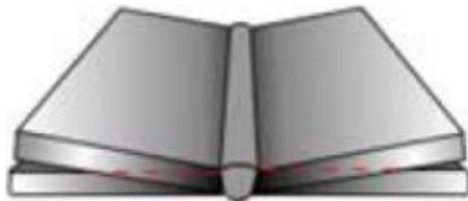
Figure 2.9 Angular distortion
