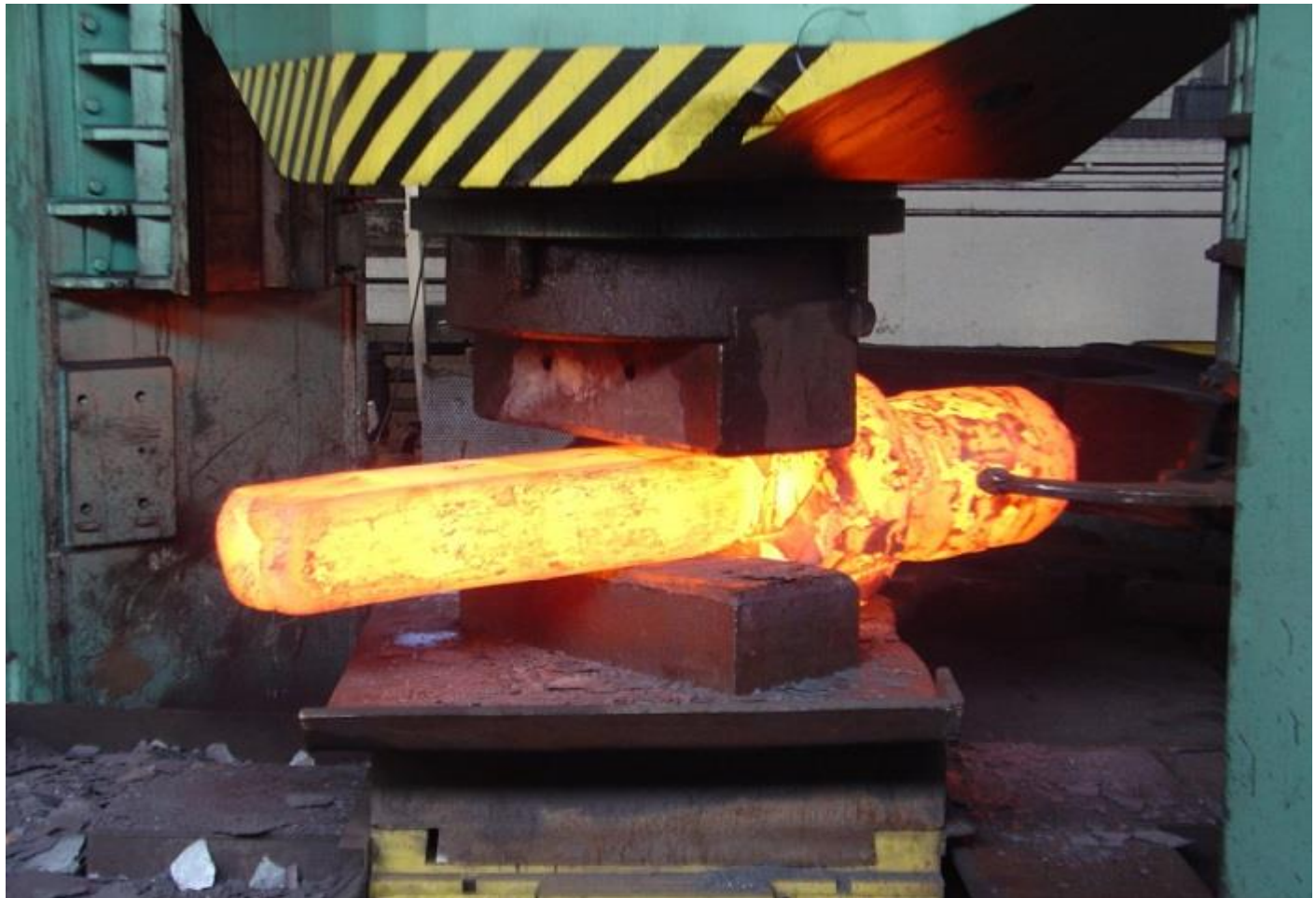
Figure 3.4 Production of Open Die Forging
