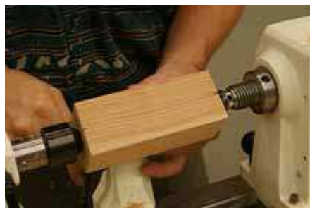
Fig. 2.56 Exercise blank mounted on lathe
