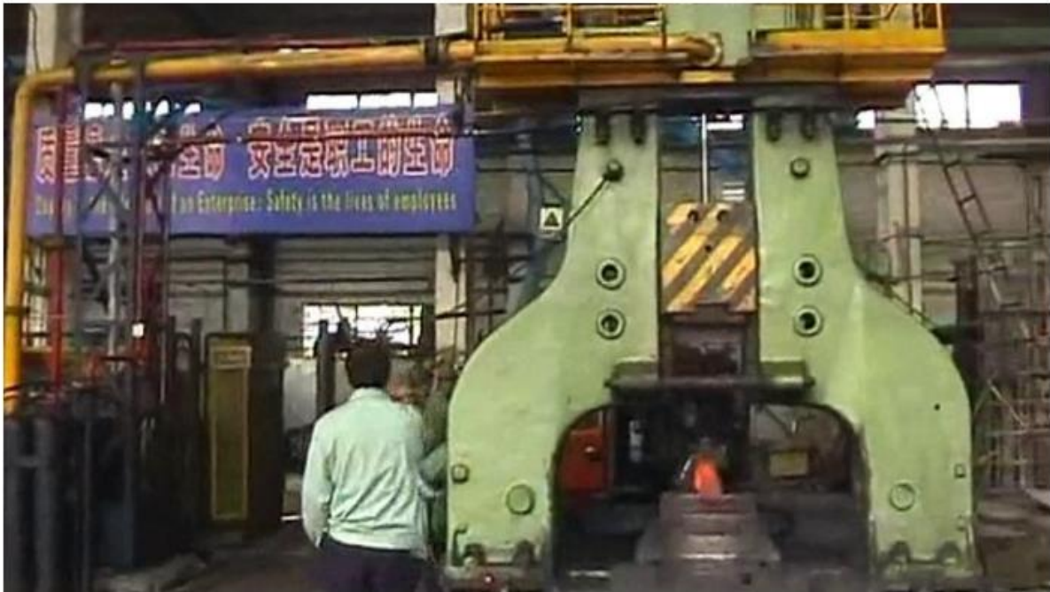
Figure 3.5 Open die forging equipment
