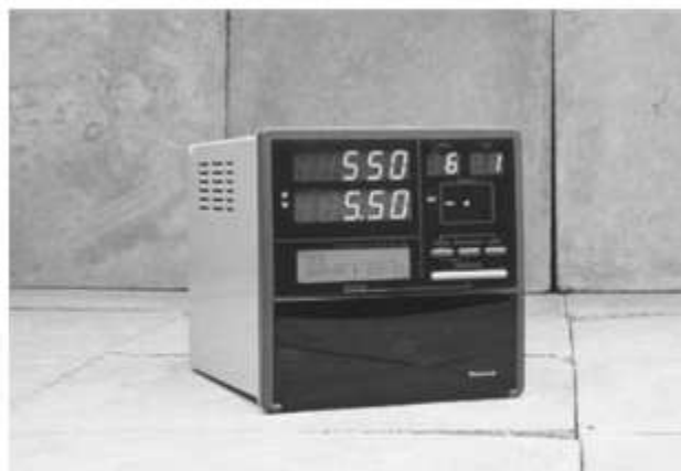
Fig.2.3 Ramp-soak, programmable, single-point temperature controller. Courtesy of Honeywell, Inc.
