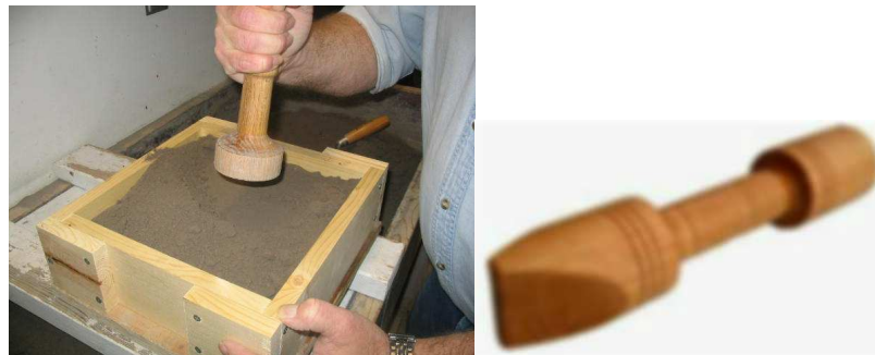
Figure 3.20 Ramming the Sand
