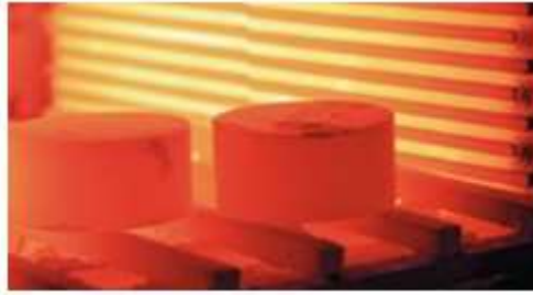
Fig.1.2 Thermal Treatments microstructure of the material or change the phase structure to improve the mechanical properties
