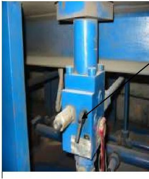
Figure 3 Arrow in the picture is showing drain valve
