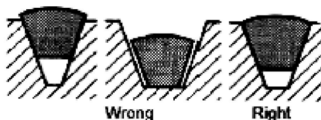
Fig. 2.4 Check if the V-belt will fit to the pulley
