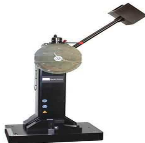
Fig. 7. Instrumented impact pendulum system for Charpy testing (courtesy of Instron)
