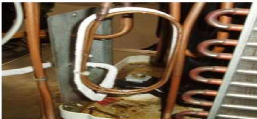
when capillary tube is clogged
