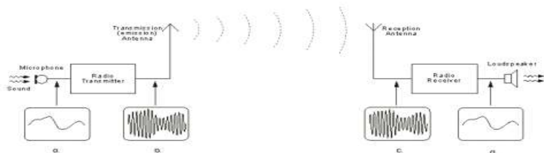
Fig. 1: Radio Communication System - Transmission and Reception
