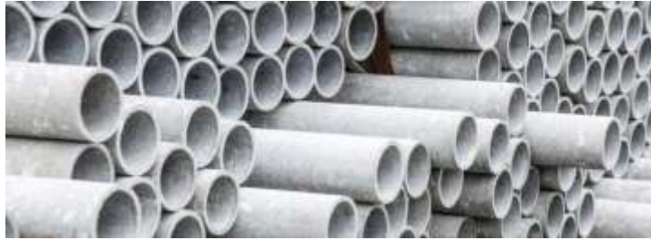
Figure 1.25 asbestos cement pipe
