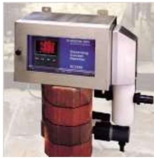
Figure 2.2. streaming current detector
