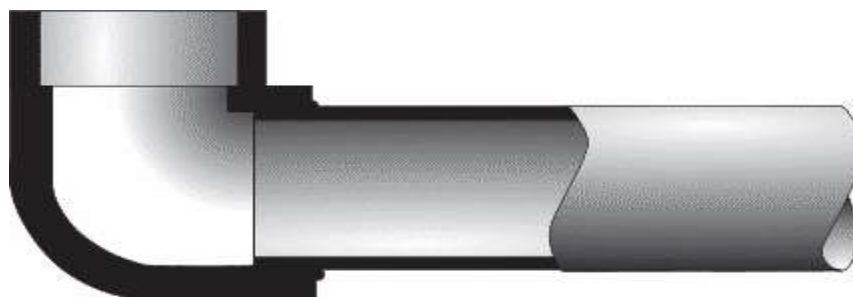
Figure 2.3 Standard Socket Fusion Joint
