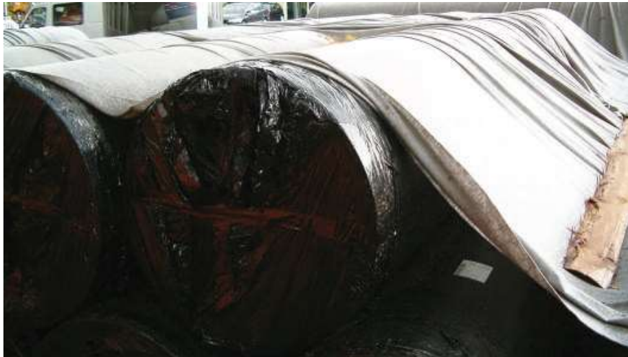
Figure 1.1 Protection of pipe against direct sunlight
