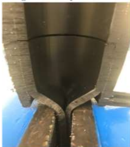
Figure 1.2b Coupling Crush Test
