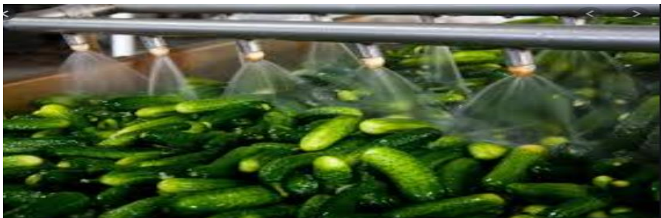
Fig 1. Cleaning vegetable product by using water spray
