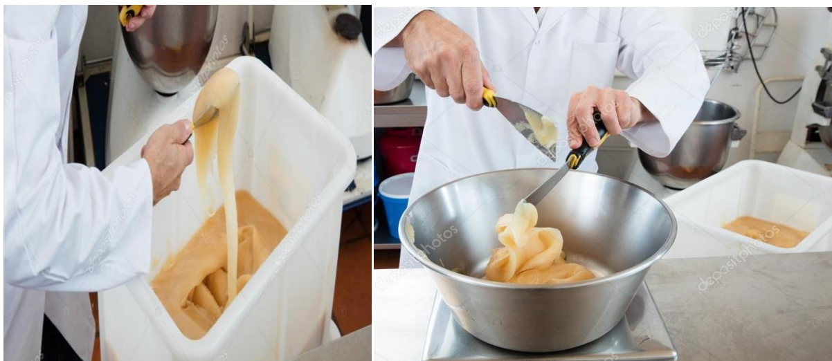
Figure 22: Weighing honey using Platform weighing balance
