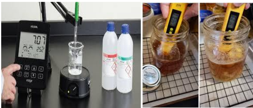
Figure 5: Calibration of pH meter and measuring pH of sample
