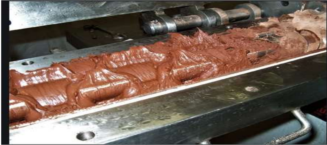
Fig 1 Conching operation process by screw mixing machine
