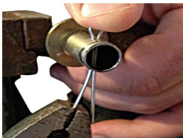
Figure 12. Grasp the long section of the cotter pin. Figure 13. Grasp the other section of the cotter pin.
