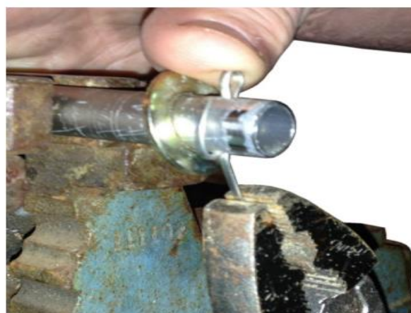
Figure 12. Grasp the long section of the cotter pin. Figure 13. Grasp the other section of the cotter pin.
