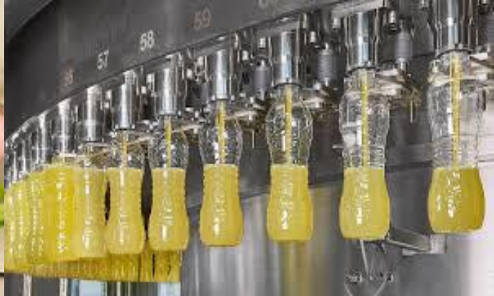
Fig: 4.2 filling bottles with juice
