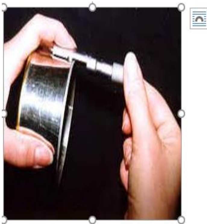
Figure 5.4: measuring a can seam
