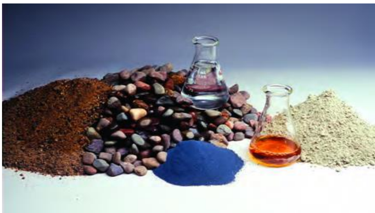
Figure 1: Concrete components: cement, water, coarse aggregate, fine aggregate, supplementary cementing materials, and chemical admixtures.
