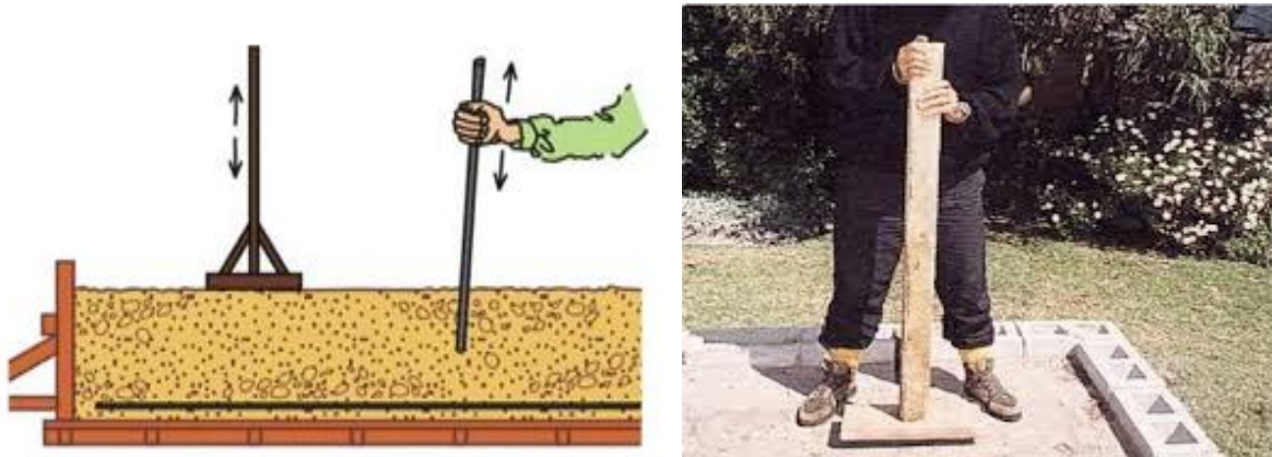
Figure 112: Concrete compacting by hand
