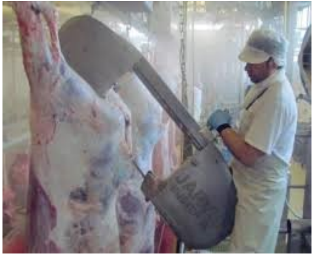
Figure 7 Electrical carcass spilling machine
