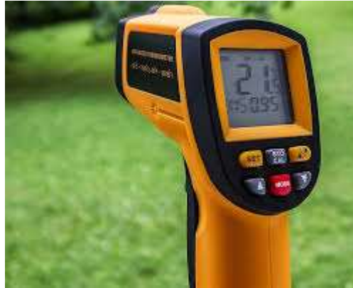
Fig1.9 Radiation /infrared thermometer
