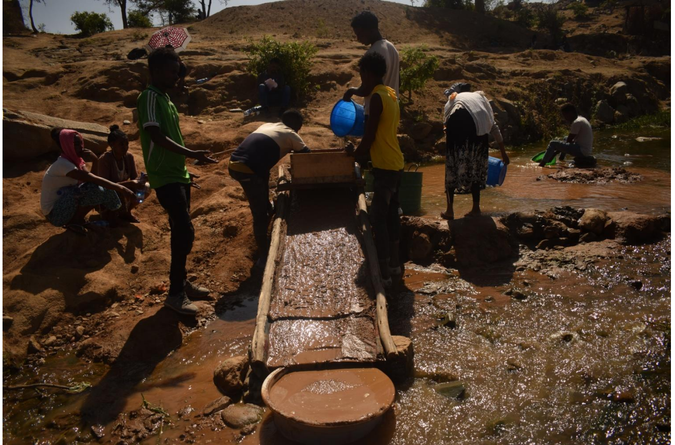
Fig1: Gold ore processing within the river using sluice box
