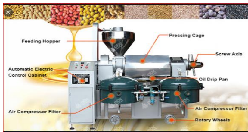
Figure 5: Material feeding or loading in hydraulic press
