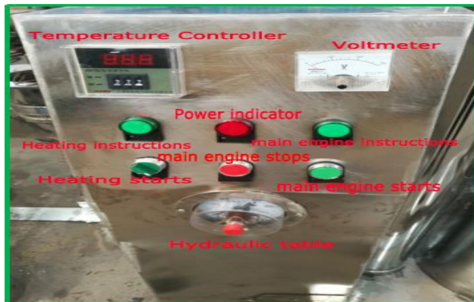
Figure 14: Operation Diagram of Hydraulic oil press machine
