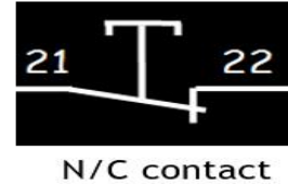
Figure 2.5 Electrical device and symbol of start and stop push button
