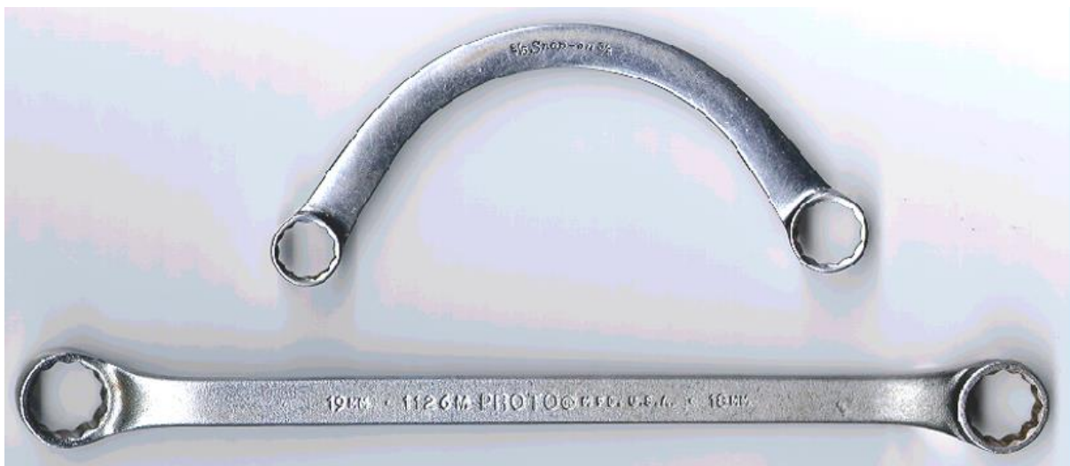
Figure 2.4 different type and size of box end wrenches
