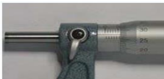
Figure 3.5. Micrometer thimble reading 5.78mm
