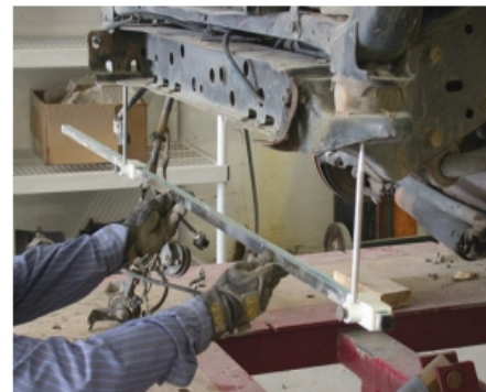
Figure 3 A tram gauge is handy when you have to measure across points on a vehicle to find major damage. Adjust the gauge to the correct dimension from the manual and then compare it to actual points on the damaged vehicle
