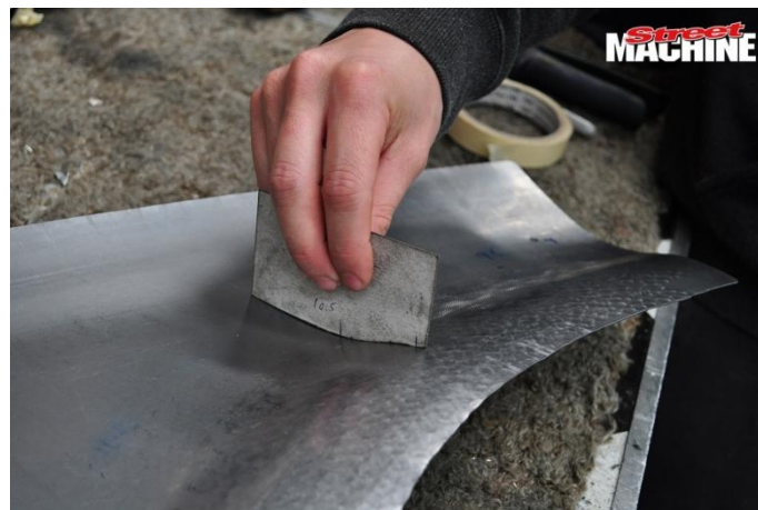
Figure 45 checking accuracy of formed sheet metal by using pattern
