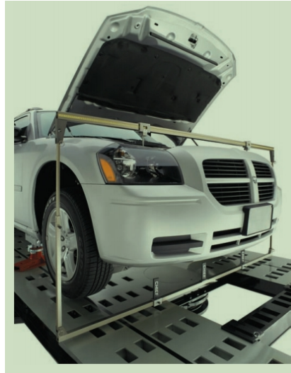
Figure 8 Here is typical strut center line gauge in place. The top of the strut towers is a common measurement point, because they are often moved out of alignment during frontal impact.
