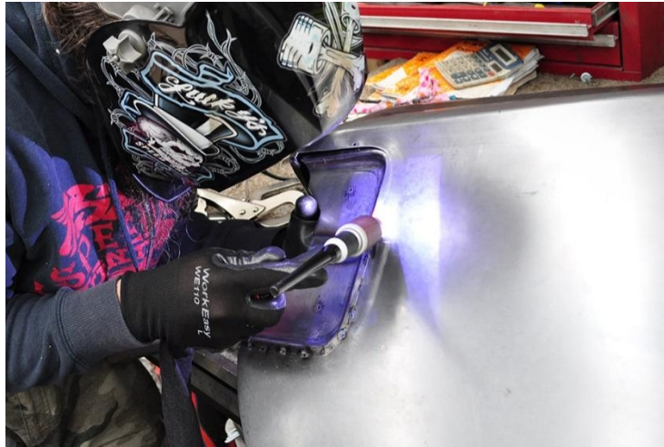
Figure 57 There's no point dumping excessive heat into the panel
