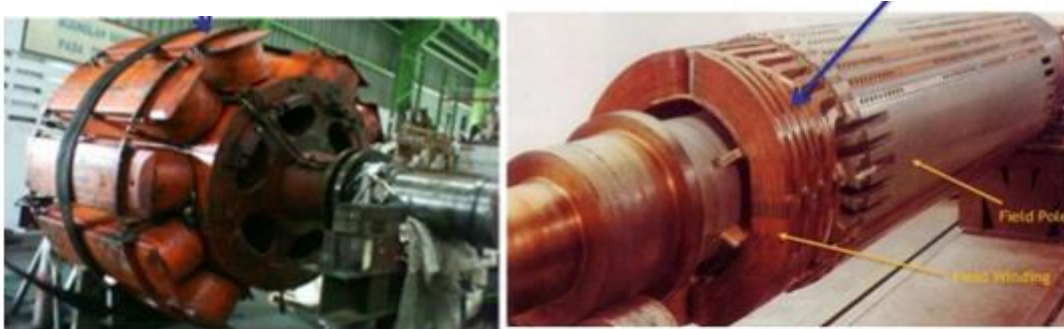
Figure 22: salient and cylindrical rotor types
