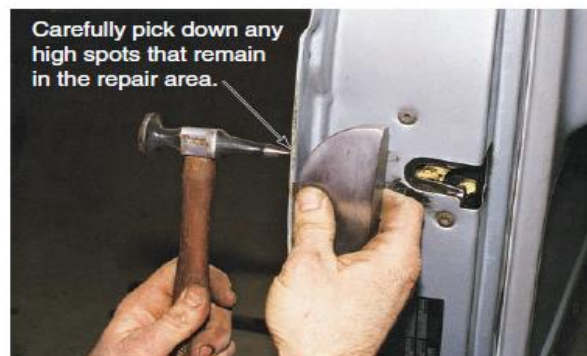
Figure 26: A pointed head or pick on a hammer is used to lower small high spots
