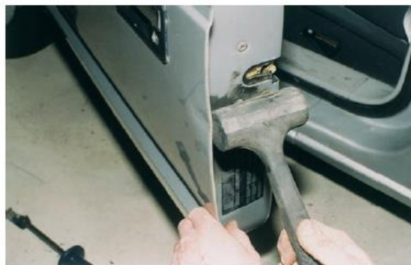
Figure 22: Remove a small dent using a plastic mallet
