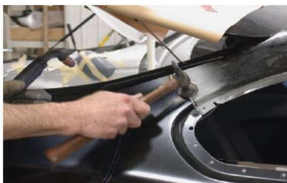
Figure 21: Body hammer to lower the sheet metal area
