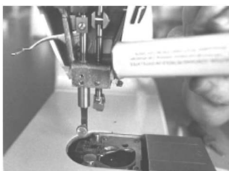
Face Plate Area—Remove lint from faceplate area using a soft brush. A cloth dipped in petrol can be used to remove grease and grime.
