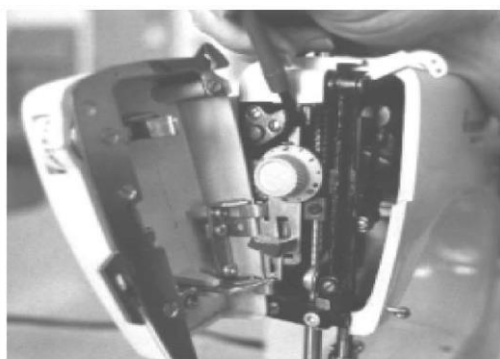
Face Plate Area—Place a drop or two of oil on moving parts where they slide through a housing or move against each other.
